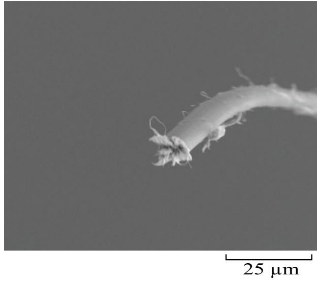
Figure 3.35: Core-shell fiber creep fracture for CS_9C ( \sigma=324 MPa, long lifetime=6051 s.).
