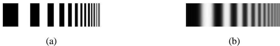
**Figure 29: (a) High contrast periodic grating and (b) Image of the high contrast periodic grating**
