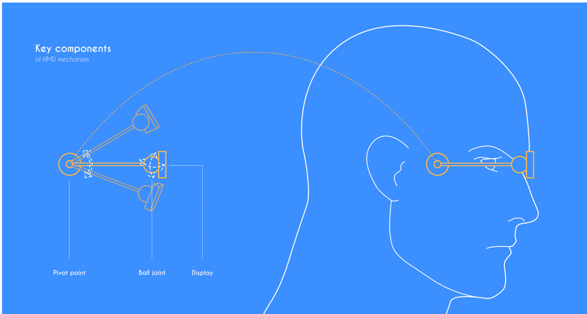
Figure 25. A concept design focusing on the mechanism for future HMD
