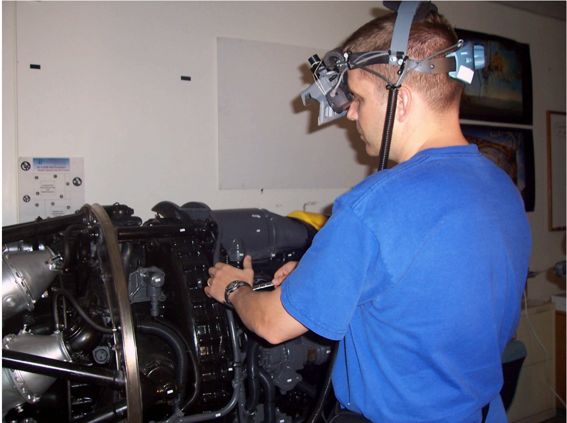
Figure 2. A mechanic wearing a tracked head-worn display performs a maintenance task on a Rolls Royce DART 510 Engine.
