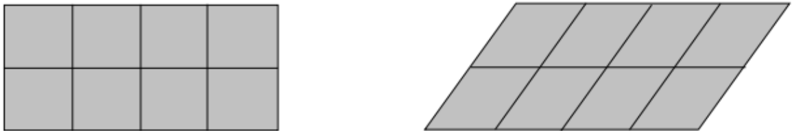
Figure 2.9. Lagrangian mesh showing how deformation of the body is deforming the mesh [15].
