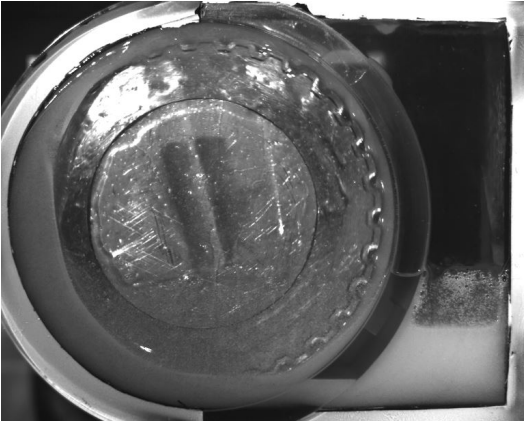
Figure 4.20. Experimental oil flow behavior after 1.5s at 250 rpm, 10mm inlet and 15mm outlet.
