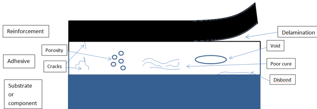
Figure 8. Various common defects in a composite [15].
