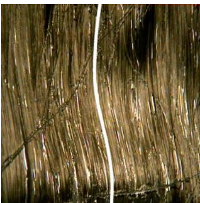
Figure 9. How fibre misalignment looks like [21].
