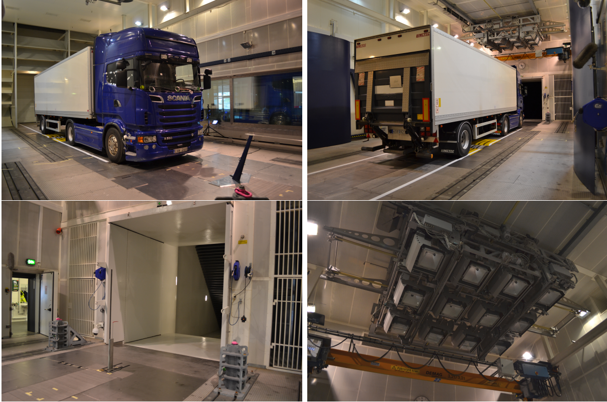
Figure 1.2: Photos inside the climatic wind tunnel from the measuring campaign. Test truck with city trailer and Prandtl-probe (top left). Truck set up from behind and nozzle (top right). Nozzle, wind tunnel access door and Prandtl-probe (bottom left). Solar lamp array in the wind tunnel ceiling (bottom right).
