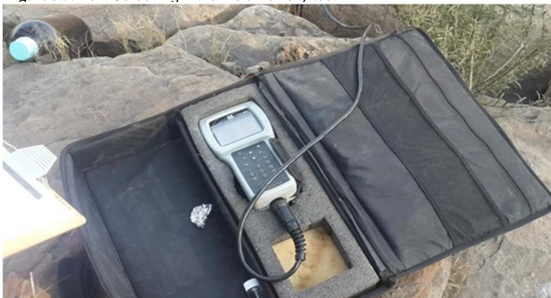
Figure 3. 6 : YSI instrument for onsite water quality measurement
