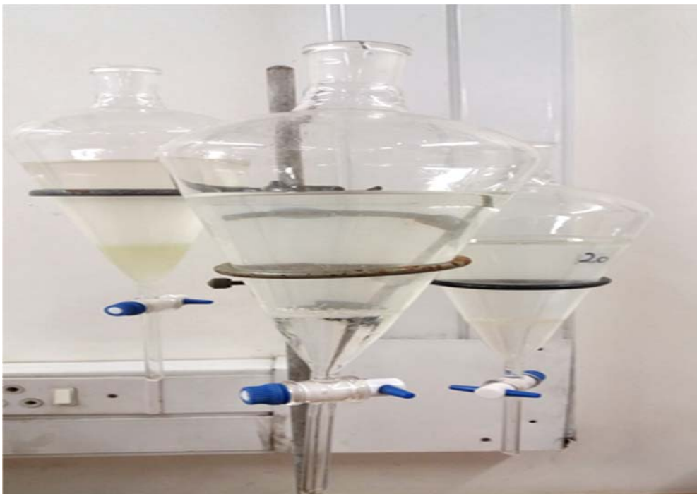
Figure 3. 2: Liquid-liquid extraction of water samples
