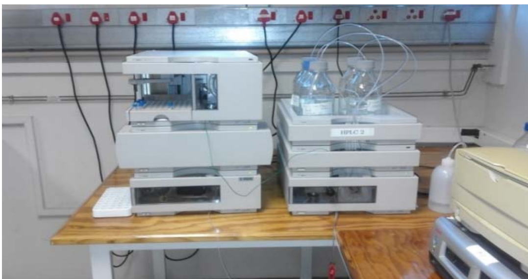
Figure 2.2: Figure showing a typical HPLC laboratory set up
