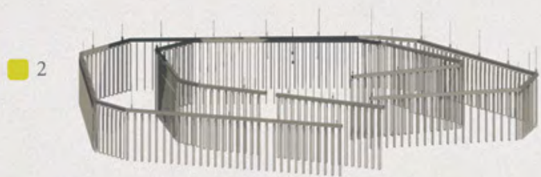
Raised Walkway Overhead Frame
