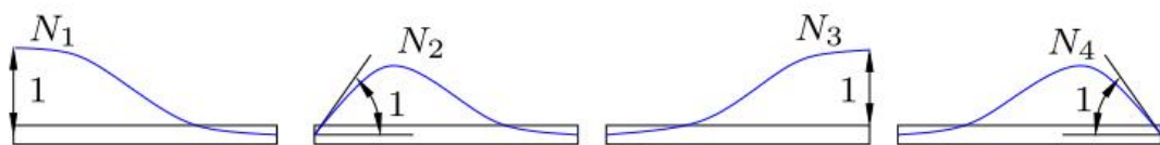
Figure 4. Example shape functions of the Euler–Bernoulli beam element (University of Oulu 2014: 15).
