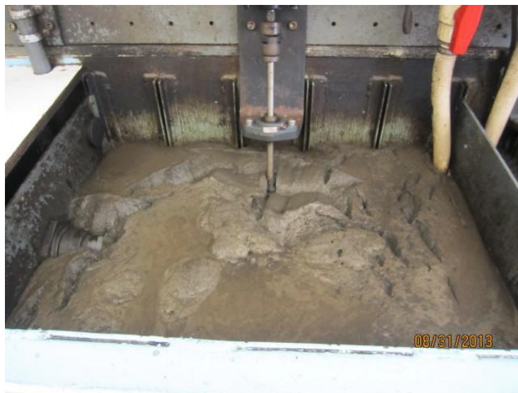
Figure 1.1 Foaming in the UBC pilot plant (MEBPR system).
