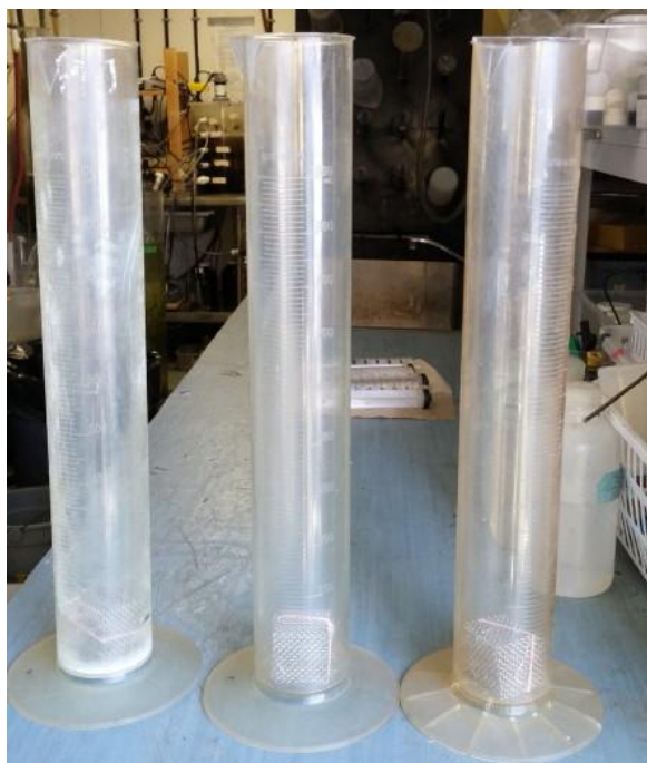
Figure 3.4 Apparatus used for foaming potential with Alka-Seltzer tablet (stainless steel cages were used to hold the tablets)
