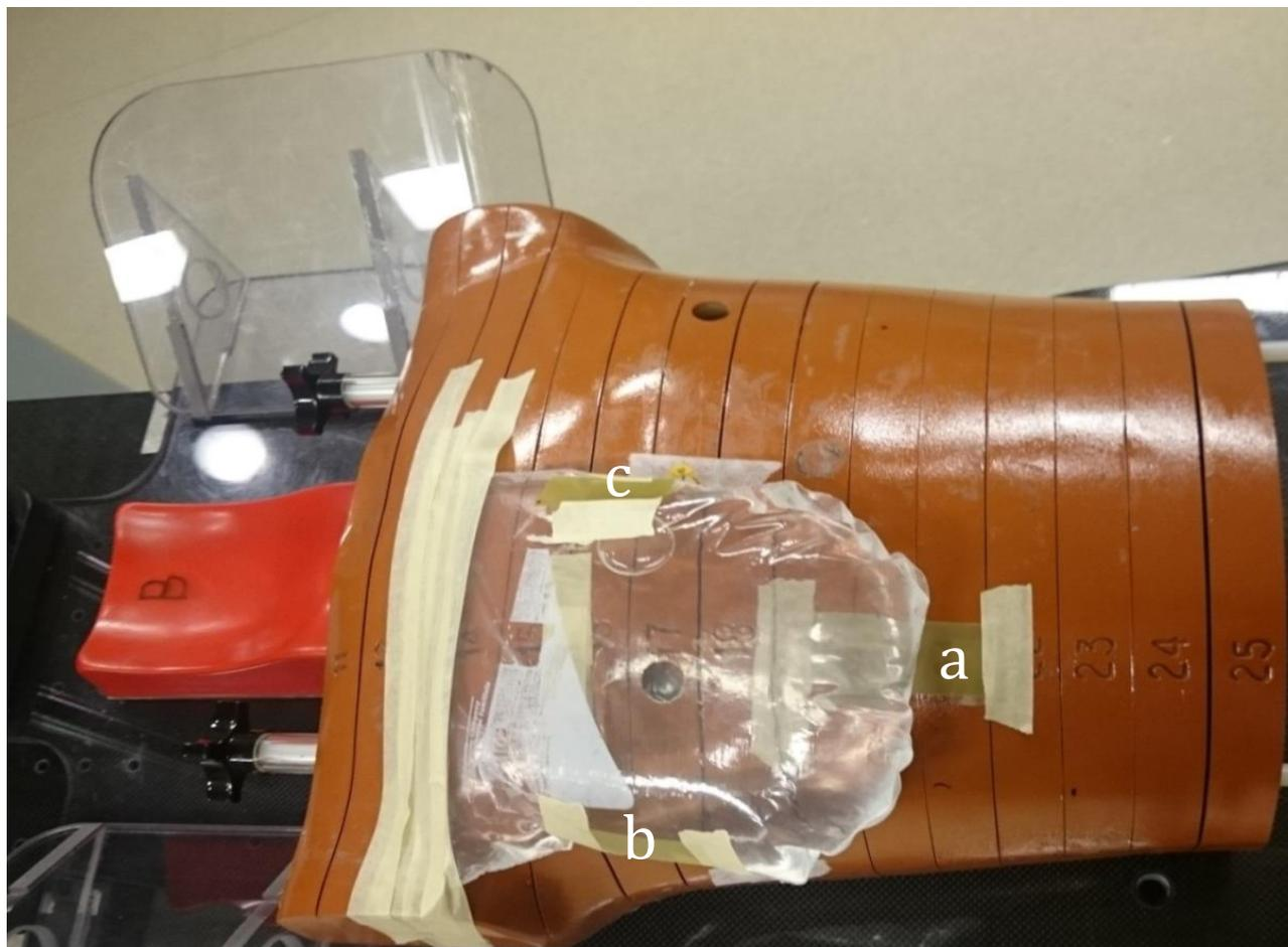
**Figure 4.3:** Photograph of the phantom set up for dose delivery using foam wedge. EBT3 film locations, (a-upper) fourth film placed under the breast above the foam wedge, (a-lower) the fifth film is also under the foam wedge on the chest surface (b), the sixth film is placed on the right (lateral) side of the phantom, (c) the seventh film is placed on the left (medial) side of the phantom.
