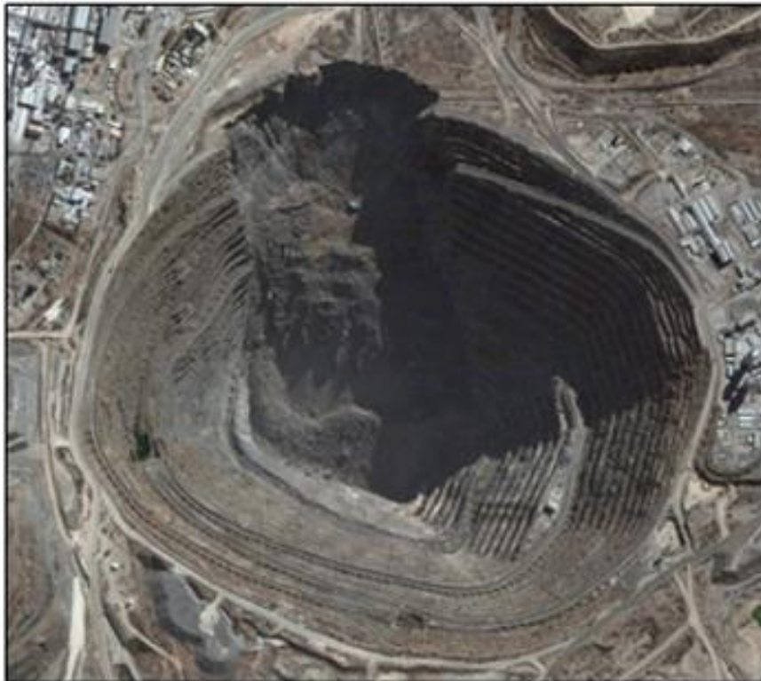
Figure 4.23. a) 3-D spatial relationship between the underground operations, open pit, and Mica Fault; and b) 2008 Quickbird image of Palabora northwest wall failure.
