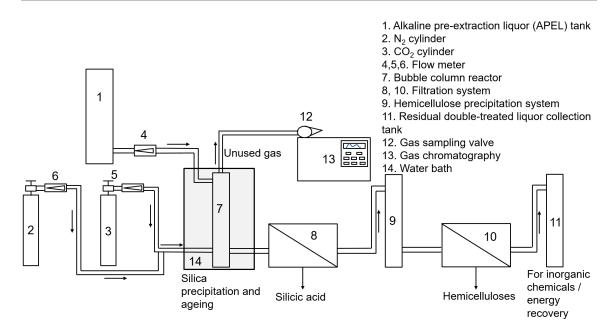
Figure 4.1: A schematic of experimental set-up for recovering silica and hemicellulose and reducing  $CO_2$  emissions.
