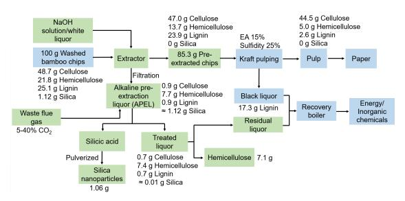
**Figure 4.9:** Proposed process of kraft pulping with extraction and recovery units of silica and hemicellulose from bamboo chips.
