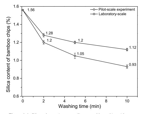
Figure A.3: Pilot-scale experiments on silica removal by washing with water.
