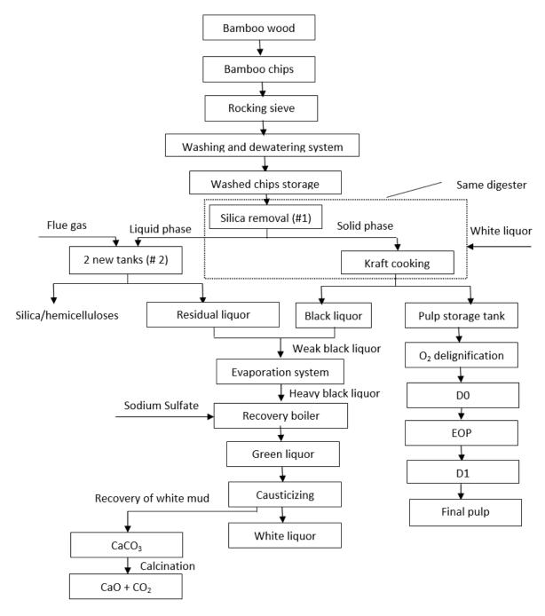
Figure 4.10: Combination of the new stages in a typical kraft bamboo pulp mill.
