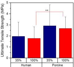
Figure 20. Tensile testing of stratum cornea to determine their in-plane mechanical properties. Orientation of tensile stress application, data collection, and analysis using a true stress-true strain plot (A); mean in-plane Young's moduli (B); and ultimate tensile strength (C) of stratum corneum from fresh human upper abdominal skin samples (n=20 across 4 human subjects), and
