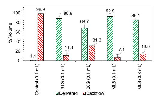
Figure 30. Comparison of ID fluid delivery methods ex vivo for successful fluid delivery and fluid backflow resulting in wastage (n=5 for the control, 31G needle, and 26G needle for 0.1 mL injections; n=6 for 0.1 mL injections using ML6; n=4 for 0.3 mL injections using ML6; error bars represent standard deviation).
