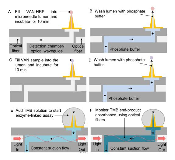
Figure 38. Process of conducting the biosensing process in the microneedle-optofluidic device. Microneedle lumens were pre-loaded with vancomycin-HRP before binding the vancomycin in an unknown sample. The enzyme-linked TMB assay was used to quantify the remaining vancomycin-HRP in the microneedle lumen surface.
