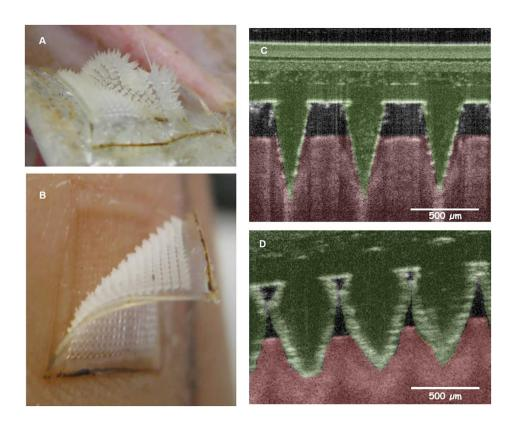
Figure 7. Hydrogel-forming microneedles for extraction of analytes from ISF [48].
