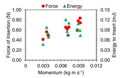
Figure 26 Impact of momentum on the insertion of a single microneedle into skin. Force and energy required to insert a single microneedle of 100  $\mu$ m outer tip diameter into the artificial skin model were determined (n=12) at a constant total energy of 1.2 mJ. The momentum was altered by changing the moving mass m of the microneedle.
