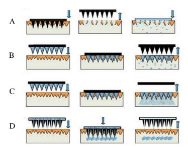
Figure 2. Common strategies for drug delivery using microneedles. (A) Solid microneedles create micro-pores in skin prior to topical drug/patch application; (B) coated solid microneedles to transfer drugs into skin; (C) dissolving solid polymeric microneedles; and (D) hollow microneedles arrays to inject drugs and extract fluids [25]. The orange layer represents the epidermis of skin, including the stratum corneum.
