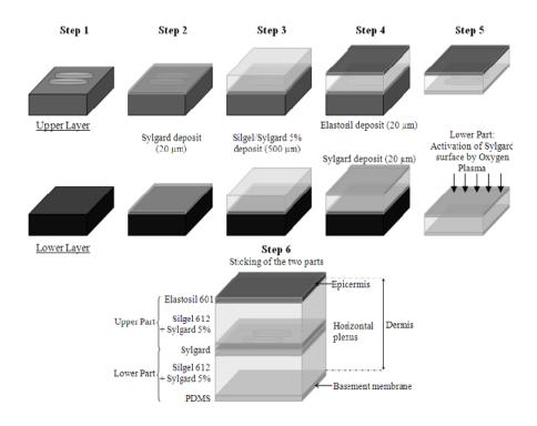
Figure 16. Soft lithography process of fabricating an artificial mechanical skin model from silicone rubber products [114].
