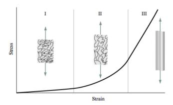
Figure 12. Stress versus strain relationship of skin resulting in a *J*-shaped curve. Regions marked I-III represent low to high modulus responses, respectively[65].
