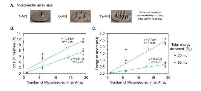
Figure 28. Impact of the number of microneedles in an array on skin insertion. (A) Microneedle array sizes used in the study consisted of 1 (1-MN), 6 (6-MN), and 19 (19-MN) projections with 100  $\mu$ m tip outer diameter. CB) Force and (C) energy required to insert microneedle arrays as a function of the number of microneedle projections in an array, measured at two levels of total energy delivered (20 and 53 mJ).
