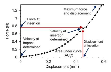
Figure 24. Microneedle insertion force versus displacement profile generated from an experiment using spring #30 (k=152 N m<sup>-1</sup>, x=4 mm, E<sub>o</sub>=1.2 mJ, and estimated v<sub>imp</sub>=0.6 m s<sup>-1</sup>) collected from the high-speed camera (at 10 kfps) and the FS01 force sensor (at 100 kHz).
