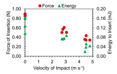
Figure 25. Factors influencing the insertion of a single microneedle into skin. Force and energy required to insert a single microneedle of outer tip diameters of 120  $\mu$ m (n=12), into the artificial skin model, as a function of the microneedle's velocity at impact against the skin.
