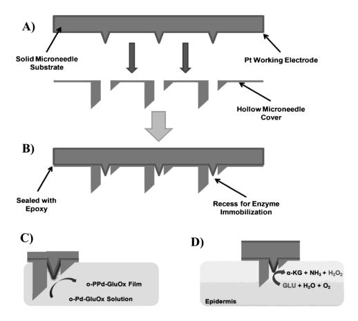
Figure 8. Bicomponent microneedle electrode system consisting of integrated hollow and solid microneedle arrays for glutamate monitoring [53].
