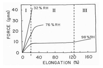
Figure 13. Tensile force versus elongation profiles for human stratum corneum at different relative humidity conditions. Regions I-III represent Hookean, yielding, and strain-hardening regions, respectively. Stratum corneum sample size was 8 mm (length) x 2 mm (width) [68].
