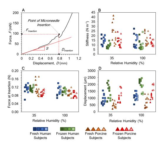
Figure 18. Microneedle insertion profiling in skin layers. (A) Force versus displacement data from a typical microneedle insertion profile was evaluated for stiffness (B), force of insertion (C), and displacement at insertion (D) parameters for human and porcine skin before and after freezing at -80 °C for 48 hours (four human and four porcine subjects tested at 35% and 100% RH; n=4 per subject per condition).
