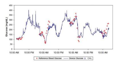
Figure 10. Continuous glucose monitoring by the microneedle biosensor compared to reference blood glucose [54].
