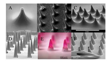
Figure 3. Arrays of solid and hollow out-of-plane microneedles. (A) Hollow silicon microneedles by deep reactive ion etching [14]; (B) solid silicon microneedles [27]; (C) clay-reinforced polyimide microneedle array by solvent casting [18]; (D) solid stainless steel microneedles by laser cutting; (E) dissolving polymeric microneedles [12]; (F) laser-machined metallic microneedle array [28].
