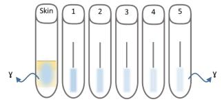
Figure 29. Fluid delivery and measurement methodology. (A) A highly dilute <sup>99m</sup>TcO<sub>4</sub>- solution is administered using ID delivery devices. (B) Fluid backflow to the skin surface post-administration is captured by cotton swabs. (C) Gamma radiation present in skin and cotton swabs is measured using a gamma counter.
