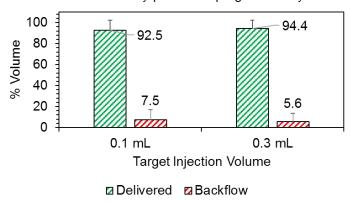
Figure 31. In vivo delivery of <sup>99m</sup>TcO<sub>4</sub> solution using the ML1 single microneedle device in Sprague Dawley rats (n=3 for the 0.1 mL injections; n=3 for 0.3 mL injections; error bars represent standard deviation).
