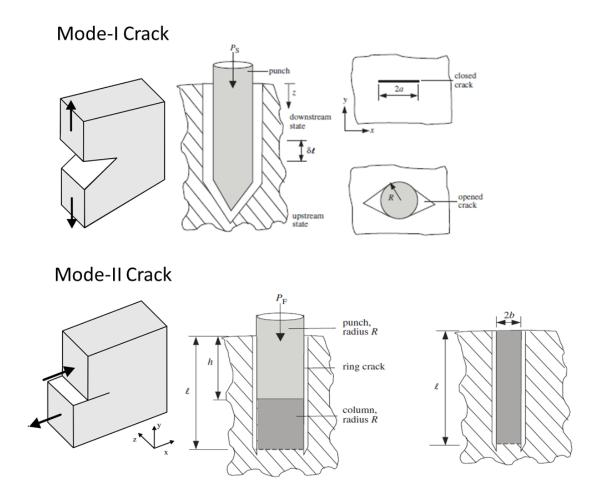
Figure 14. Penetration mechanism of soft solids by a sharp-tipped punch/needle leading to a mode-I crack and a flat-tipped punch/needle leading to a mode II crack and a compressed column of tissue [82].
