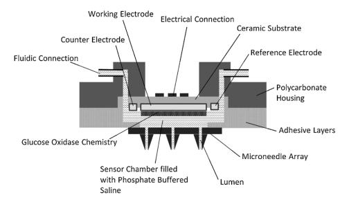
Figure 9. Continuous glucose monitoring biosensor [55].
