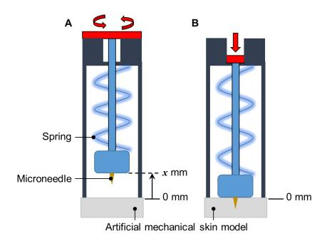
Figure 23. Dynamic microneedle insertion steps. (A) The spring inside the insertion device is compressed to a pre-defined level (x) to input energy into the system and locked in position by a rotation mechanism. (B) The spring is released by rotation causing microneedle actuation on to the artificial mechanical skin model.
