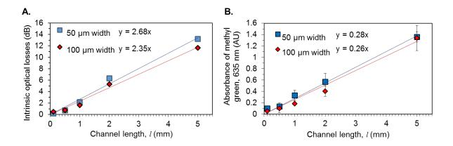
Figure 34. Optimization of the optofluidic device. (A) The width and length dimensions of the OFD waveguide were modified and tested for intrinsic optical losses using citrate buffer. (B) The absorbance of 0.001 vol% methyl green dye in absorbance units (AU), a TMB oxidation-product simulant, as a function of channel dimensions.
