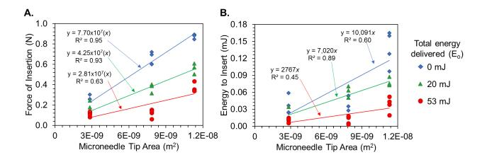
Figure 27. Impact of microneedle tip area on skin insertion. (A) Force and (E) energy required to insert a single microneedle as a function of the microneedle tip area at three levels of total energy delivered ( $E_0$ =0, 20, and 53 mJ).
