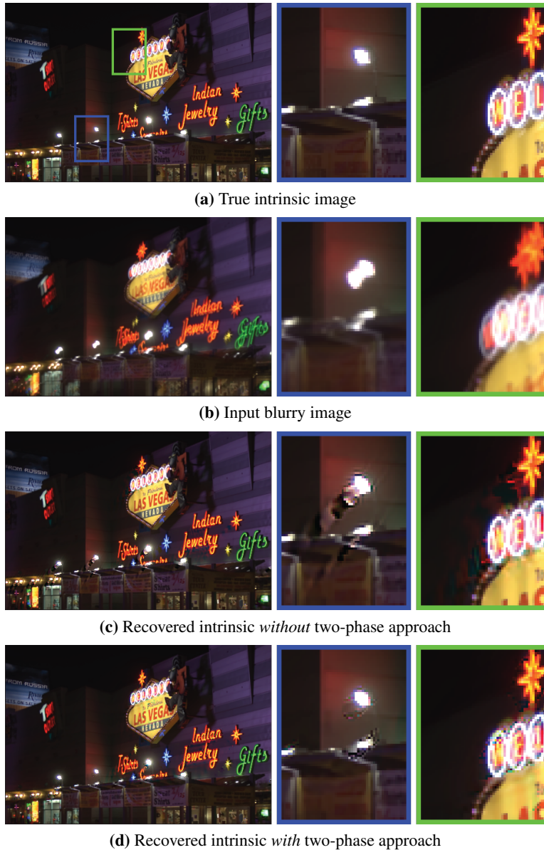
Figure 4.12: Results on partially saturated image. The dynamic range of pixel intensities in the true intrinsic image is [0, 68] . The simulated blurry image is clamped to 1. The proposed two-phase approach helps reduce ringing artifacts near saturated pixels.
