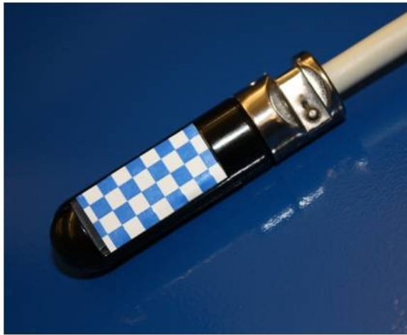
Figure 1.9: Top: Diagram showing the cross section of the “pick-up” transducer, and the location of the electromagnetic (EM) sensor and crystal stack. Bottom: a photograph of the ultrasound transducer, with checkerboards used for camera tracking.
