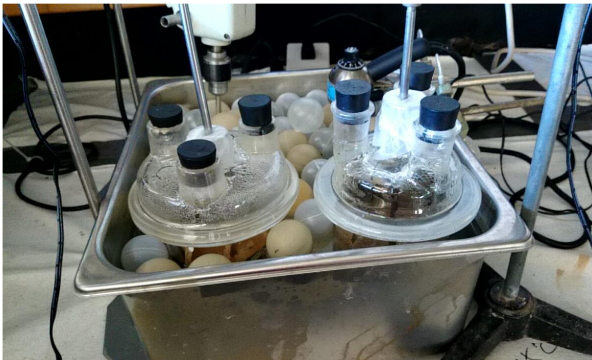
Figure 3.7 Experimental setup of leaching tank
