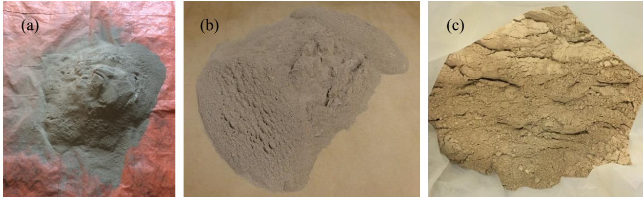
Figure 3.1 Appearance of ore samples (a) Loma de la Plata Master Composite (LDLPMC) (b) Navidad Hill Master Composite (NHMC) and (c) Connector Zone Master Composite (CZMC)
