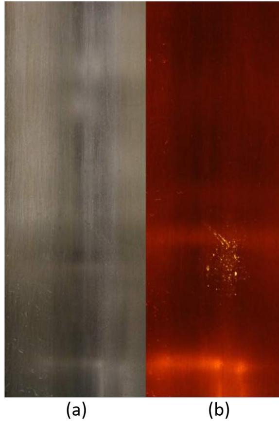
Figure 4.12: KELTRACK® transferred from wheel to rail after 1,091 m. (a) Ambient light. (b) Fluorescence.
