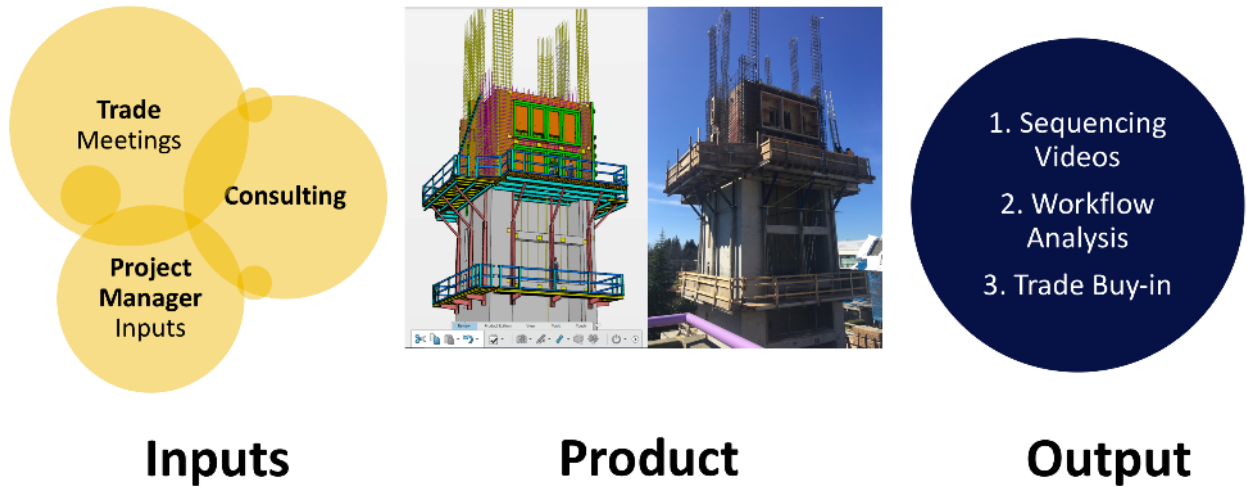
Figure 6-21 Inputs, products and outputs of the VDC model during construction and mock-up phase
