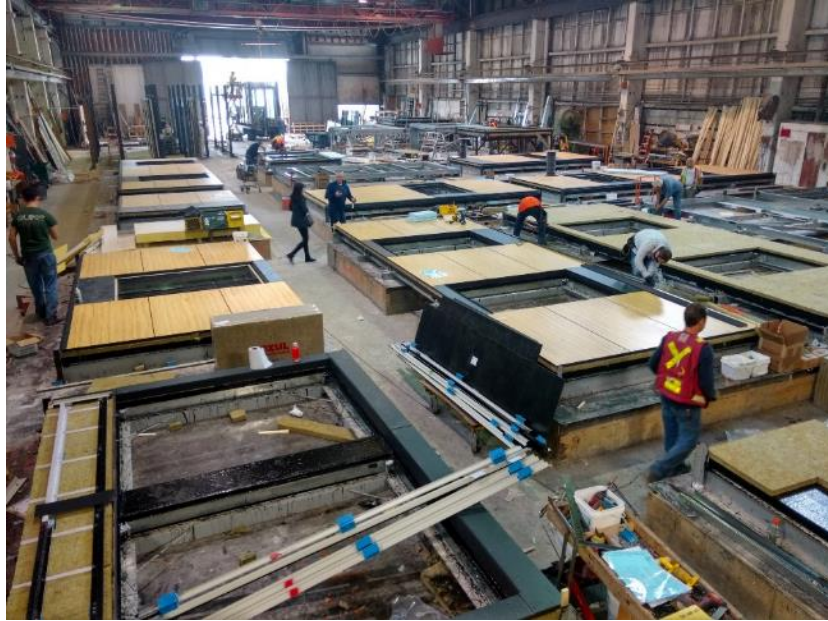
Figure 5-9 Envelope plant, jigs fixed onto the floor, for each different panel type
