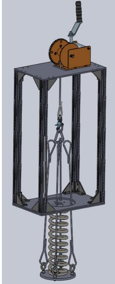
Figure 27: 3D model of the final design for the spring control mechanism
