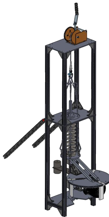
Figure 17: A 3D rendering of the final impact apparatus design.
