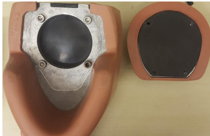
Figure 44: Custom gaskets made to keep moisture from entering the headform during on-slope testing
