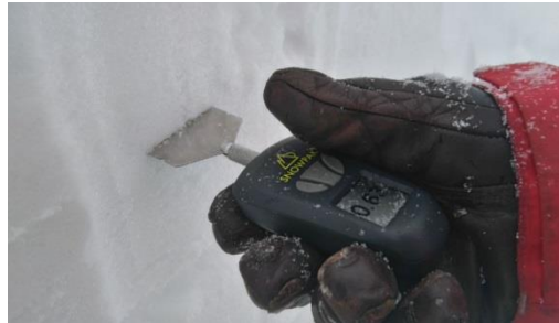
Figure 41: Demonstration of the SnowPak tool to measure the snow hardness as different snow layers. Image taken from www.snowpak.net .
