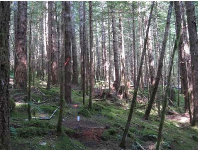
Figure 29. This image shows a static non-steady state chamber between two large trees with the chamber lid on during a site greenhouse gas flux measurement campaign.
