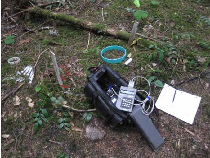
Figure 30. This image shows the ancillary GS3 instrument in use for surface soil electrical conductivity ( $EC_s$ ), volumetric water content and temperature measurements in close proximity to a static non-steady state chamber collar. Also seen are 5 vials used for greenhouse gas sample storage in preparation for chamber flux measurements.
