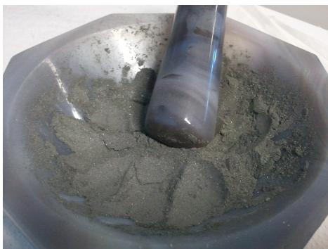
Figure 4.1: Mortar and pestle premixing
