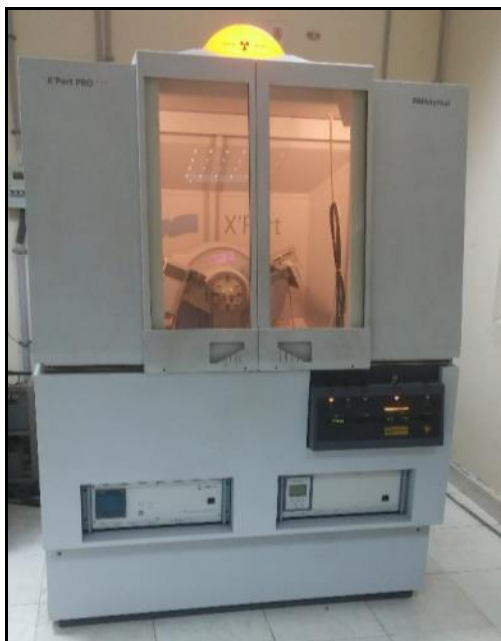
Figure 3.12: X-ray Diffractometer at IIT Chennai, India.
