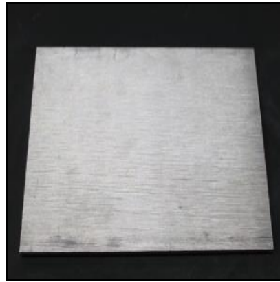
Figure 3.1: Virgin AZ31 magnesium alloy plate.
