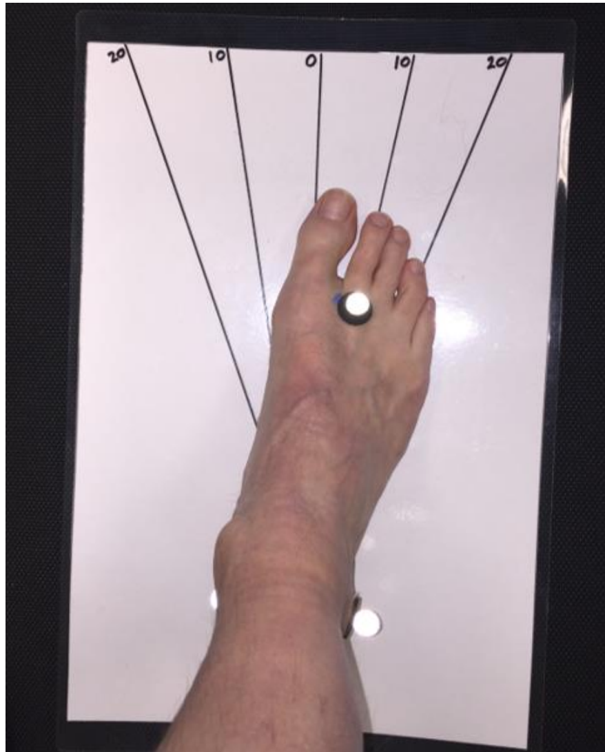
Figure 3.3: Foot placement on the protractor. The foot was placed on the protractor in line with the given condition's required foot rotation angle. The foot rotation angle magnitude while the foot was in this position was then used to determine the guideline position on screen to direct treadmill training.
