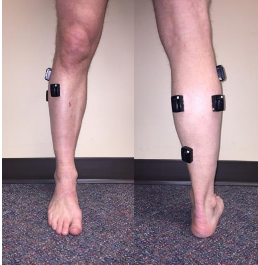
Figure 3.2: Wireless electrode placement. Five wireless electrodes were affixed to the skin over the muscle bellies of five lower leg muscles. Tape was then utilized to secure the electrodes in place (not shown, for clarity).
