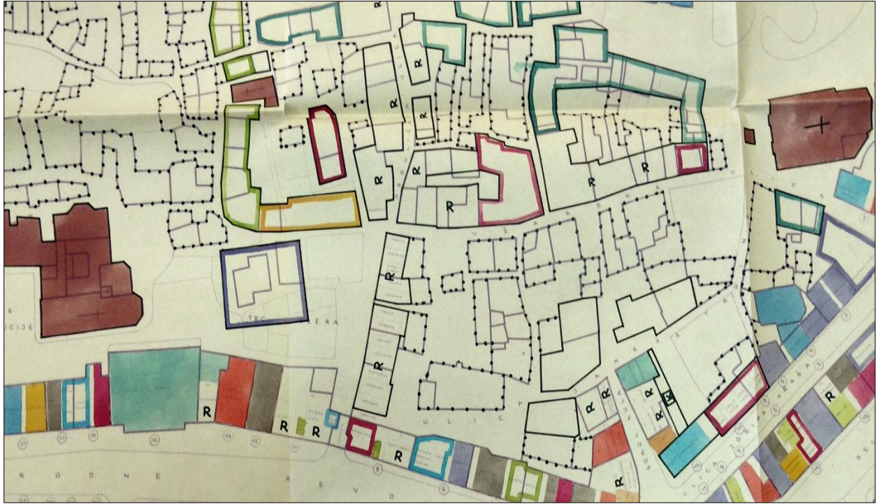
Figure 40. The street grid in a part of the northern, older belt in downtown Rijeka. The streets are very narrow, thus reducing the air circulation 336
