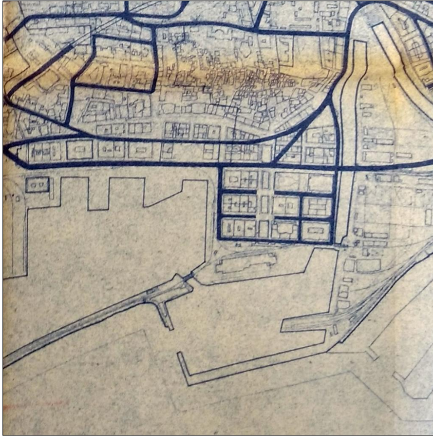
Figure 32. Proposed reconstruction of the road system in Rijeka's urban core. Two major east-west axes were proposed to improve the traffic conditions (in the center of the image). Also, the streets surrounding the city marketplace were to be expanded (in the bottom-right corner) 291
