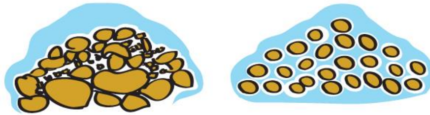
Figure 2.9 – Effect of sizing on fluid dispersion and wetting. The figure depicts the difference when ores in a heap leach operation are not subject to a crushing and agglomeration (left) and when they (right). By subjecting an ore to crushing and agglomeration extraction leach kinetics can be improved as there is more uniformity of acid to ore surface. Fines in the ore reduce extraction kinetics due to localized saturation. Agglomeration helps bind the fines into larger particles, increasing heap permeability and reducing the limitations caused by fines. ©(Captaine & Carlson, 2017)
