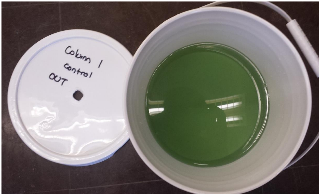
Figure 3.9 – Pregnant Leach Solution in output reservoir collection buckets. The PLS samples were collected in buckets as shown in the picture above. The weight of the collected sample was recorded daily. A sample of the solution was also collected to determine copper concentration. The dark green color is the result of the easily reachable copper being leached first. The color of the collected fluid becomes lighter over time as leachable copper in the ore gradually diminishes.
