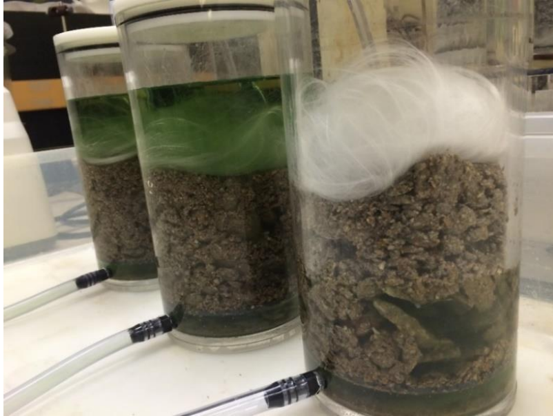
Figure 3.8 - Flooded VAT columns with leach flow upward through column. The picture shows the columns during the first few hours of leaching. The deep rich green color results from the dissolution of copper from the agglomeration stage. Pregnant leach solution exited from the top of the column.
