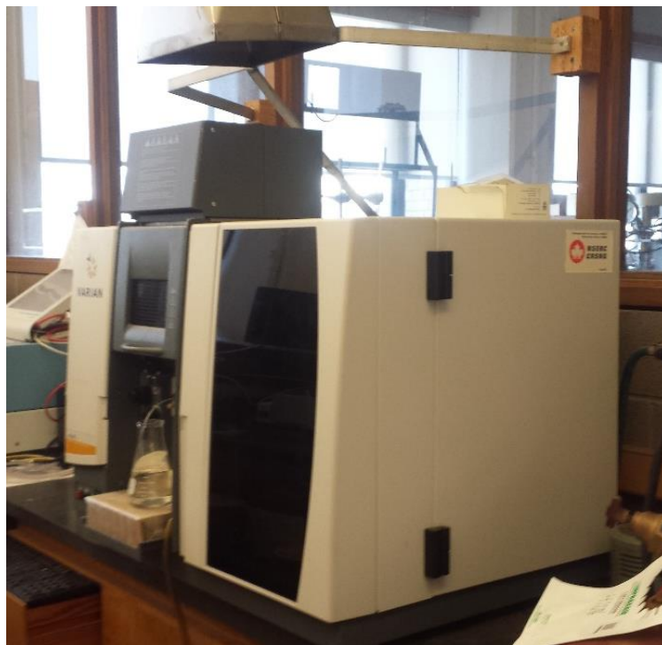
Figure 3.10 – Varian AAS 240 Atomic Absorbance Spectrometer
