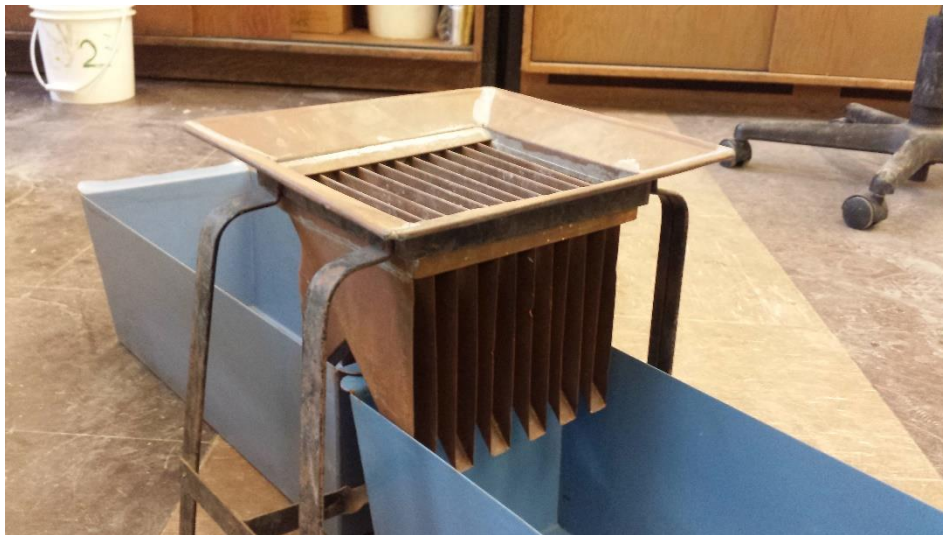
Figure 5.10 – Mechanical Riffle Splitter. The riffle splitter provides an easy and convenient way to split a bulk sample of aggregate in half. Bulk sample is fed via the use of a hopper at the top. The sample is split in half as the aggregate flowing through it flows into receptacles on either side of the riffle. The standard developed by ASTM for splitting samples provides a convenient way to produce test size samples of an aggregate material that have the characteristics of the larger bulk it was split from.
