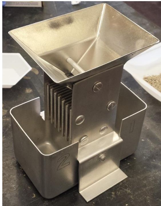
Figure 5.13 – Micro-Riffler for Sample Splitting. A micro-riffler was used to split the test charges down to sub-charges for the packed beds. A riffle split was used because in each test charge there were particles of different sizes and phases present in the mixture. The riffle splitter provided an easy way to split and randomize the produced samples. Samples fed into the hopper had an equal probability of flowing out of either discharge chute. This ensured randomization of the split samples.
