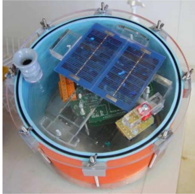
Figure 1.2: Static Wireless Sensor Node [18].
