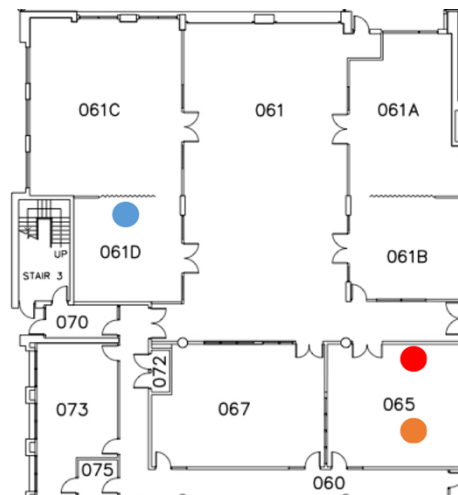
Figure 2.9: Sensor Node, Local Server and Gateway Deployment in the ICICS Building.
