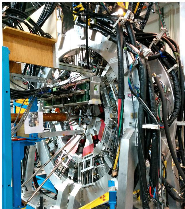
Figure 2.9: Detector arrangement used for this experiment. TIGRESS can be seen in high efficiency mode surrounding the target chamber, which contains SHARC. The mounted pre-amp rack and cabling setup, suspended above the beam line adjacent to TIGRESS, is also visible in this photograph.
