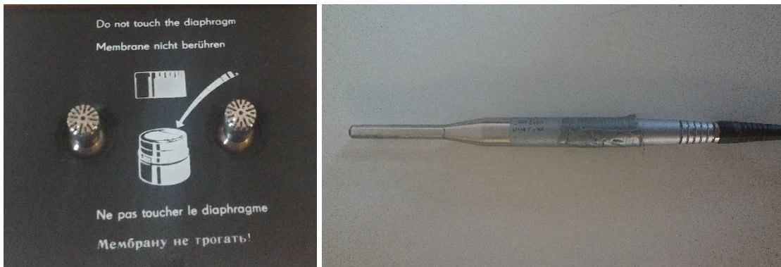
Figure 25. A pair of Phase Matched B&K 4178 Microphones and B&K 2269 Preamplifier with 1/2 inch to 1/4 inch Adapter..
