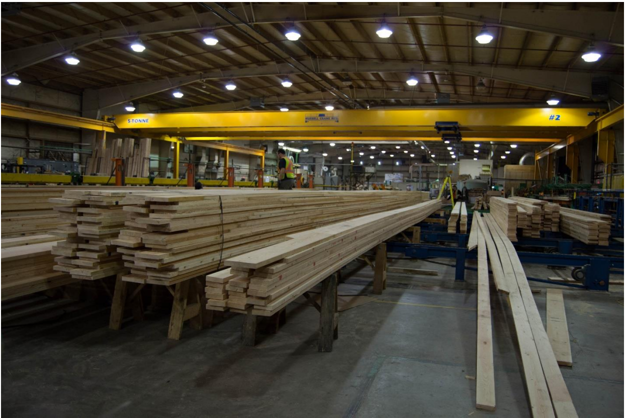
Figure 8. Material Preparation Station for CLT and Glulam in Structurlam.
