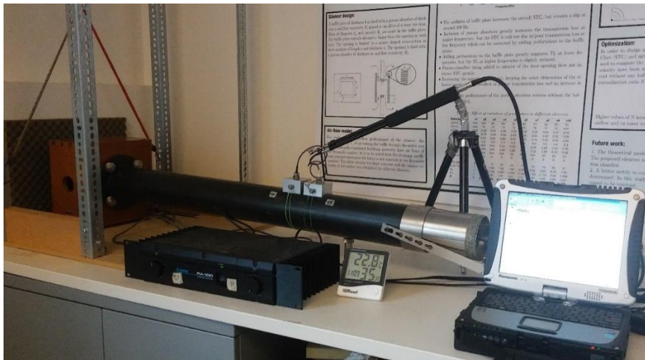
Figure 26. Low-Frequency Impedance Tube and Power Amplifier.
