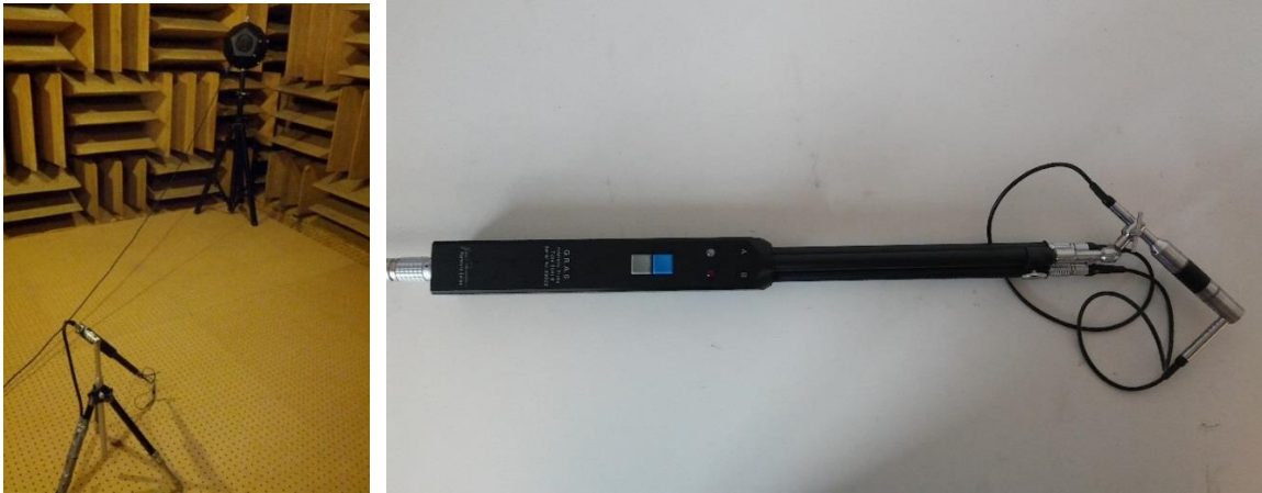
Figure 28. Spherical-Decoupling Experimental Setup with GRAS Intensity Probe inside an Anechoic Chamber.
