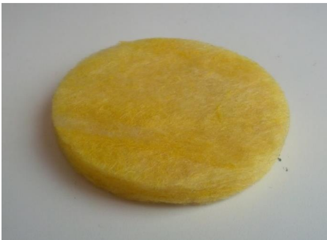
Figure 35. Sonoflex with 12.5 mm Thickness.
