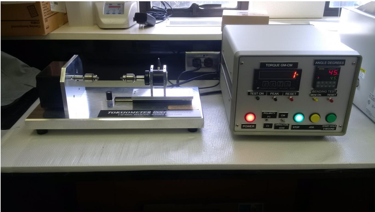
Figure 10 - Equipment to measure torsional resistance.
