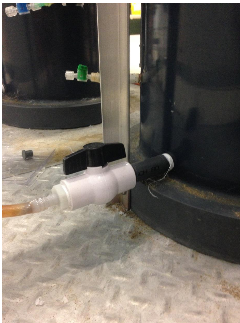
Figure 2-2 Column Base. Drainage port fitted with a PVC ball valve and connected to Tygon® tubing which makes up the manometer.
