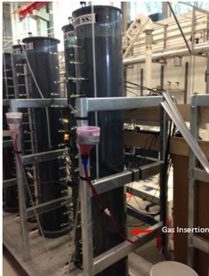
Figure 2-14 Fuels being injected using a gravity assisted method. Fuels from reservoir drain into the column through the infiltration coil.
