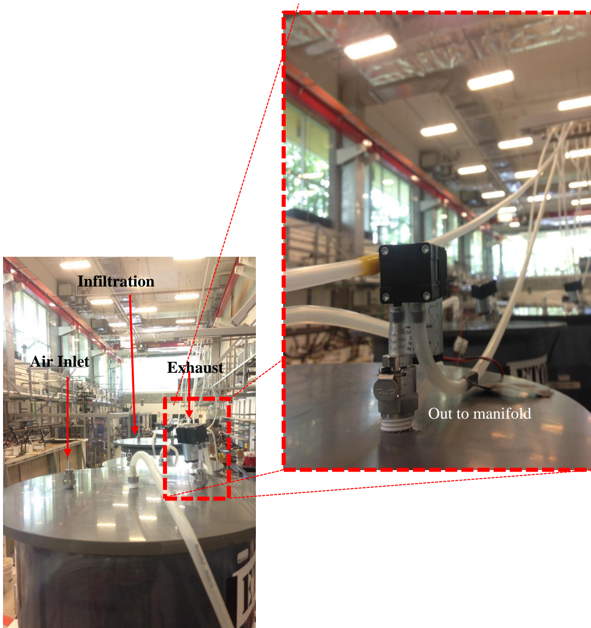
Figure 2-3 Column cap equipped with the headspace air circulation unit, and an infiltration coil which connects externally to Tygon ® tubing for optional delivery of water. A close-up of the exhaust line shows the diaphragm pump that pulls air into the column headspace and delivers the exhaust to a manifold system which leads to a fume hood.
