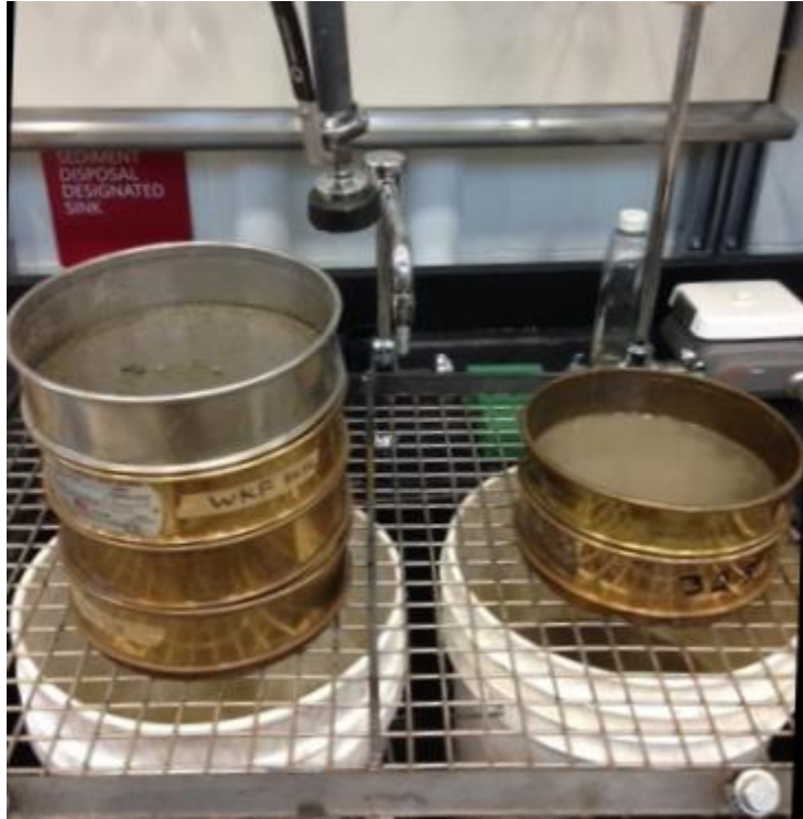
Figure 2-8 Wet sieving of sediments prior to filling of columns
