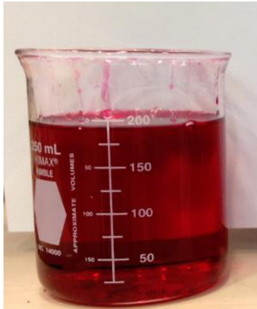
Figure 2-12 Shell V-power Nitro amended with 100mg/L Sudan IV dye. The dye aided in the visualization of the gasoline within the column
