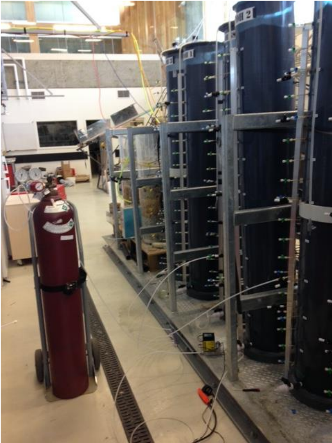
Figure D-4 Gas injection test. A gas of known composition is injected into the column at each sensor level.
