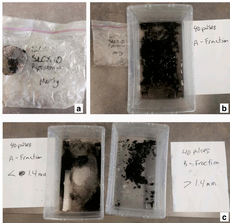
**Figure 30 SLCX processing photos.** a) sample as received. b) sample after 'gentle' 40 pulses. c) sample after sieving. 'B' fraction was then subjected to a 'harder' additional 120 pulses. Photos were taken by Daniel Layton-Mathews, Queen's University.
