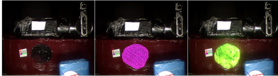
Figure 5.7: Un-augmented cross-section of phantom (left). Computer graphics overlay of tumour model (right). LPOV perspective projection of model.
