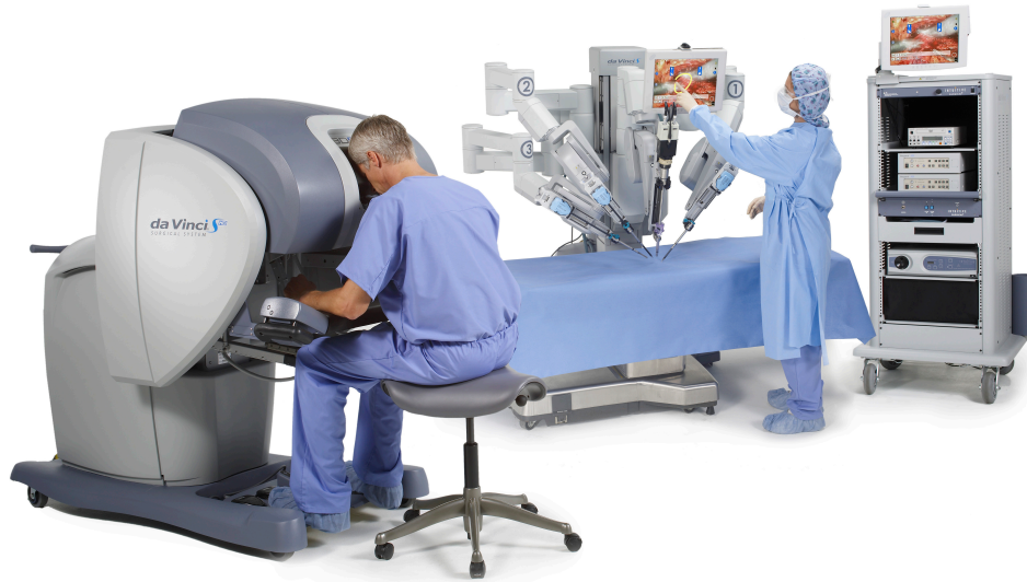
Figure 1.3: The da Vinci S Surgical System ® . The surgeon's console (left), the patient-side cart (middle), and vision cart (right). ©2017 Intuitive Surgical, Inc.
