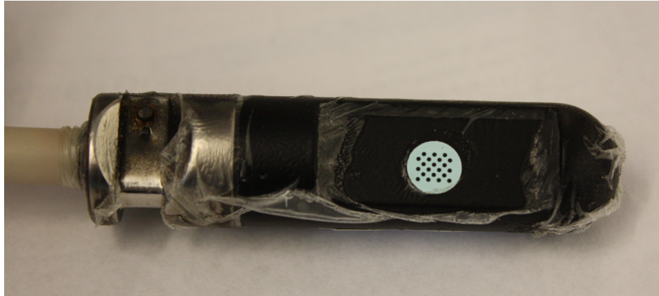
Figure 3.2: The custom “pick up” US transducer used in this work from Schneider et al.. Adhered is the tracked KeyDot ® .
