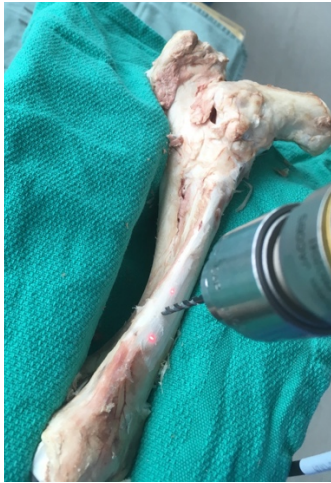
Figure 36 - Porcine femur in drilling test
