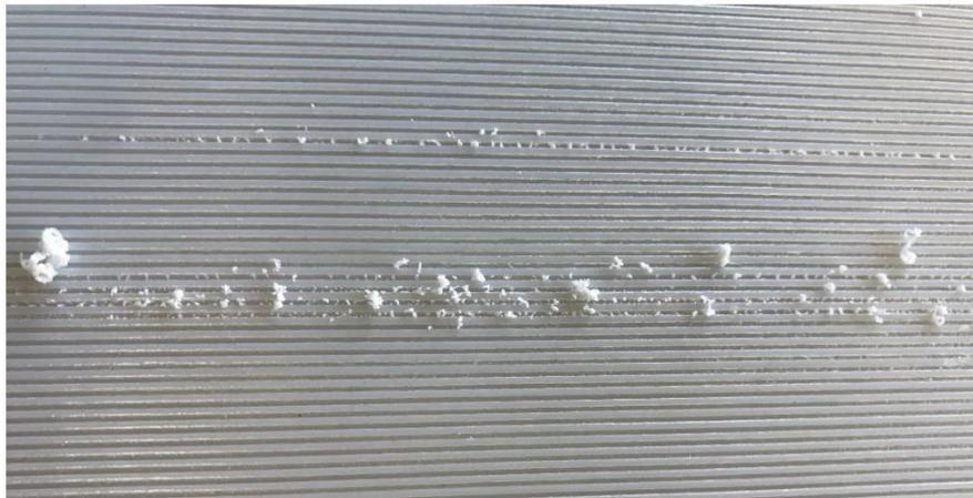
(a) Polyjet 3D printed cathode plate, clogged support materials.
