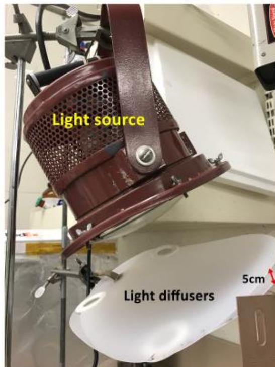
*Figure 3-7: lightening system applied for uniform lightening with constant light intensity.*
