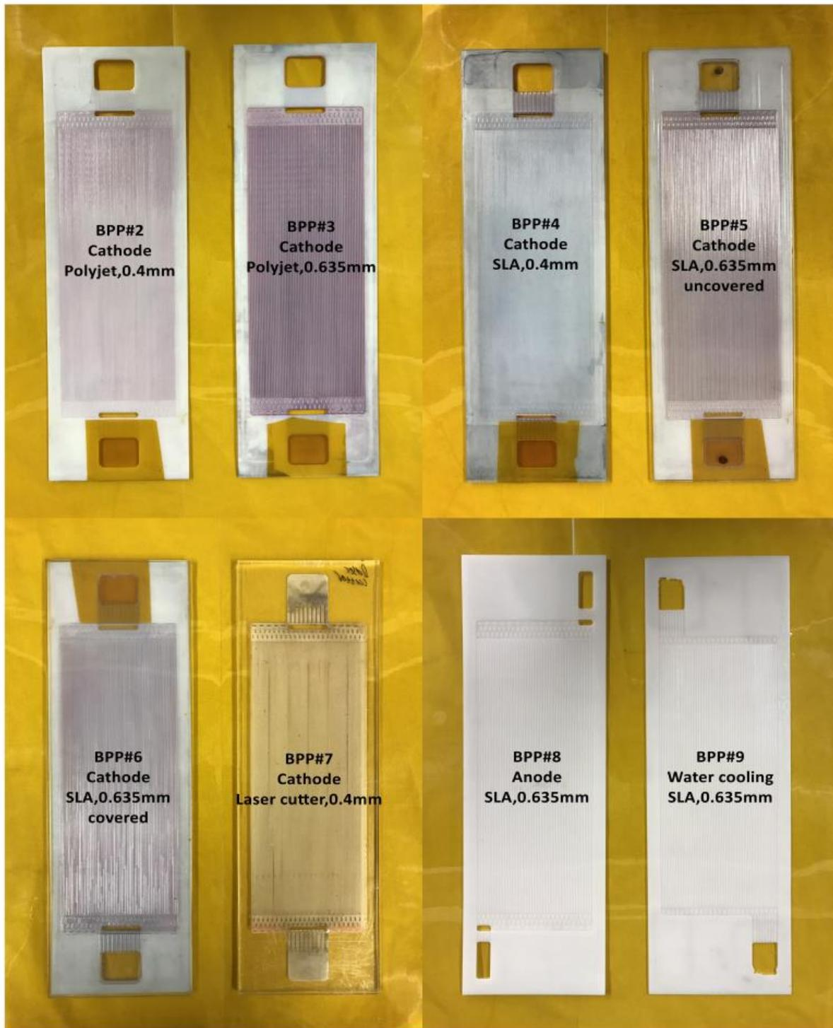
Figure 3-3: Prototype BPPs studied in the current research.
