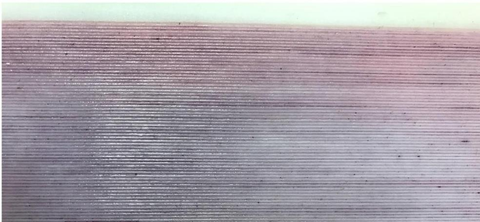
**(c) Polyjet 3D printed BPP colored with dyed water.**
