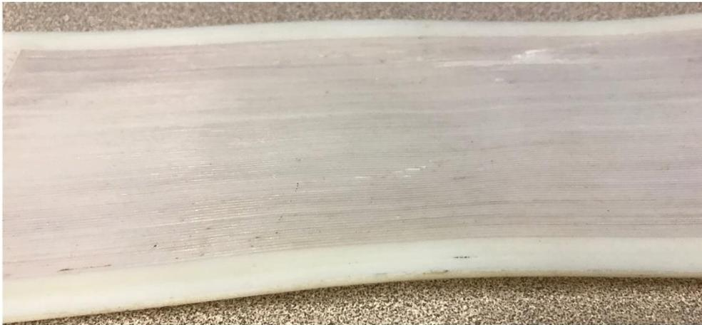
**(b) Deformed polyjet 3D printed BPP.**
