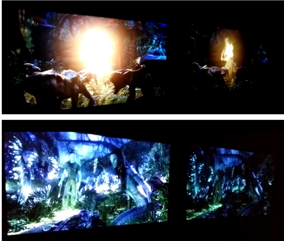
Figure 7.22: Two scenes from the movie Avatar by 20th Century FOX (top and bottom) displayed on the light steering prototype (left) and on a traditional projector with same power out of lens (right). The light steering projector (left) exceeds the comparison projector contrast and peak luminance significantly by about a factor of 20 (light steering projector: 1,000 \text{ cd/m}^2 ; right projector: 48 \text{ cd/m}^2 ).
