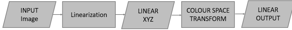
Figure 7.15: Input transformation block takes PQ-XYZ inputs, linearizes them and transforms them to the light steering projector colour space.
