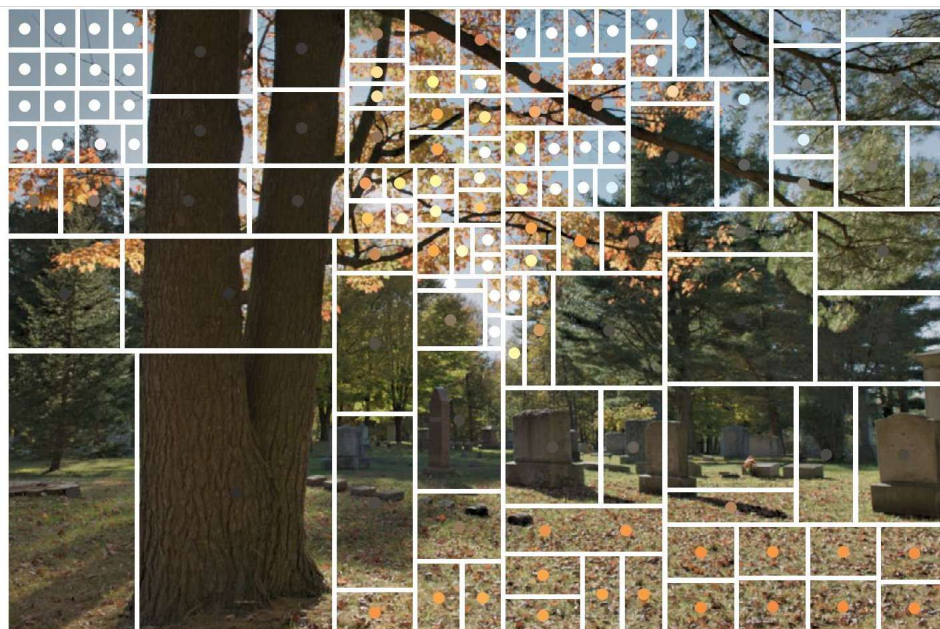
Figure 3.5: A visualization of the median cut algorithm [22], creating regions which can be represented with a single point acting as its representative light source.
