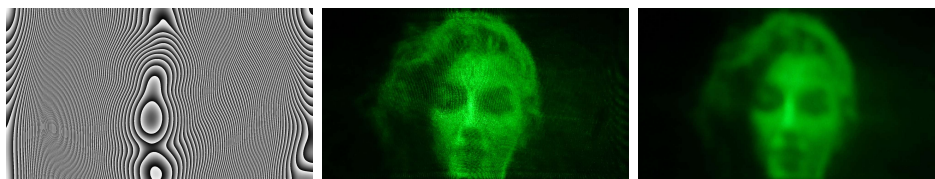
Figure 6.13: From left to right correlating to positions A to C in Figure 6.14: A: phase pattern present at phase-only LCoS modulator, B: direct image produced by lens in intermediary image plane (prior to diffuser) and C: intensity distribution present at amplitude LCoS modulator after having passed through a thin-film diffuser.
