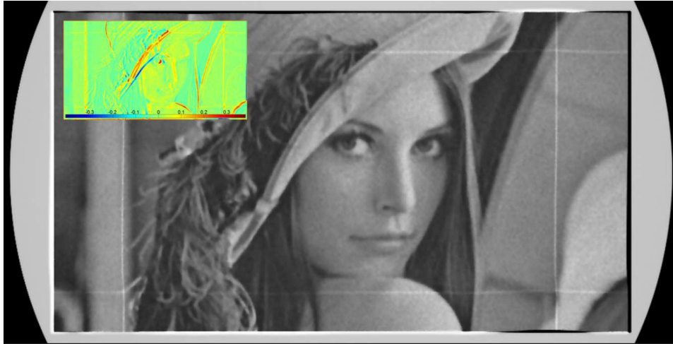
Figure 6.4: LuxRender simulation results of a caustic image caused by an acrylic freeform lens. The inset shows the absolute intensity difference between simulated and original image, where the original image is encoded in the interval [0-1], and 0 in the difference map (green) means no difference. There are three possible sources of error: reflections off the edges of the physically thick lens (vertical and horizontal lines), misalignment and scaling of the output relative to the original (manual alignment) and the nature of the light source (not perfectly collimated).
