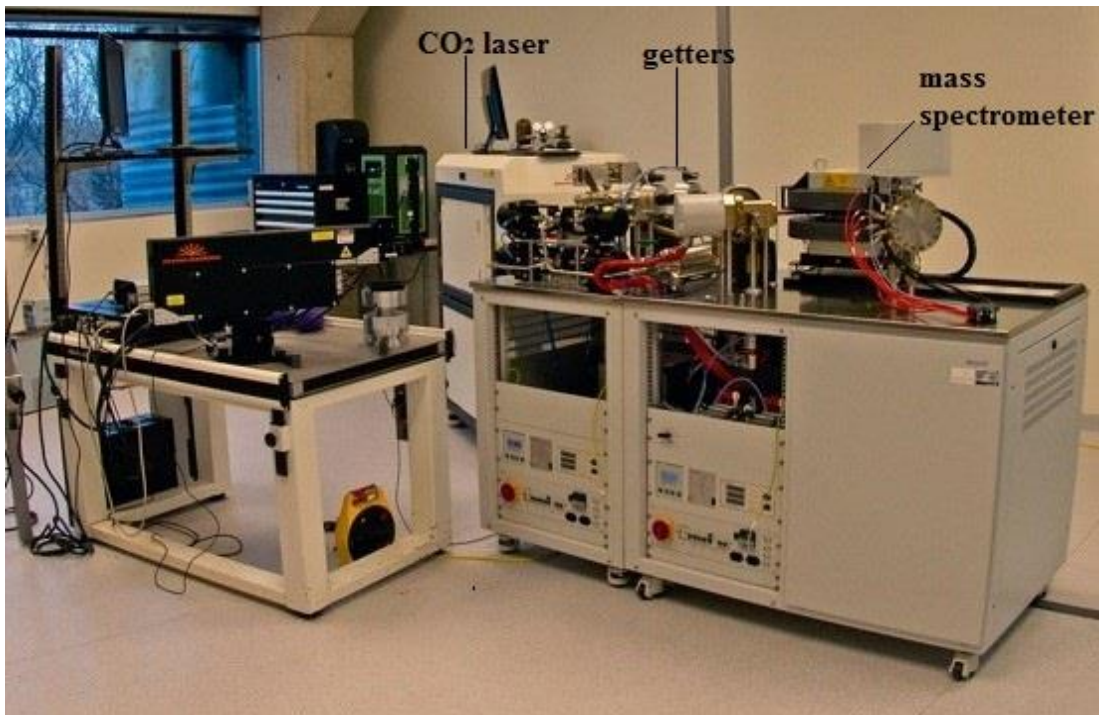
Figure 2.3. Instrument setup for ^{40}\text{Ar}^*/^{39}\text{Ar} analysis at University of Manitoba including Photon Machines CO 2 laser, SAES getters, and Argus VI mass spectrometer.
