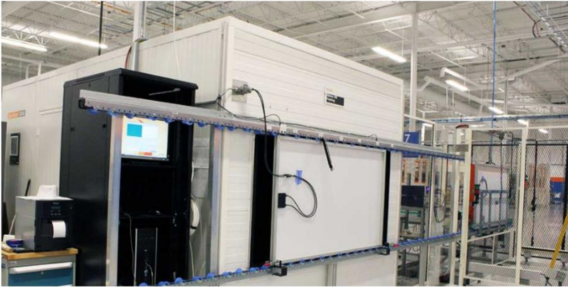
Figure 2.16: A flash tester (Class AAA solar simulator) measuring the current-voltage characteristics of photovoltaic devices. The online version of this figure is in color.
