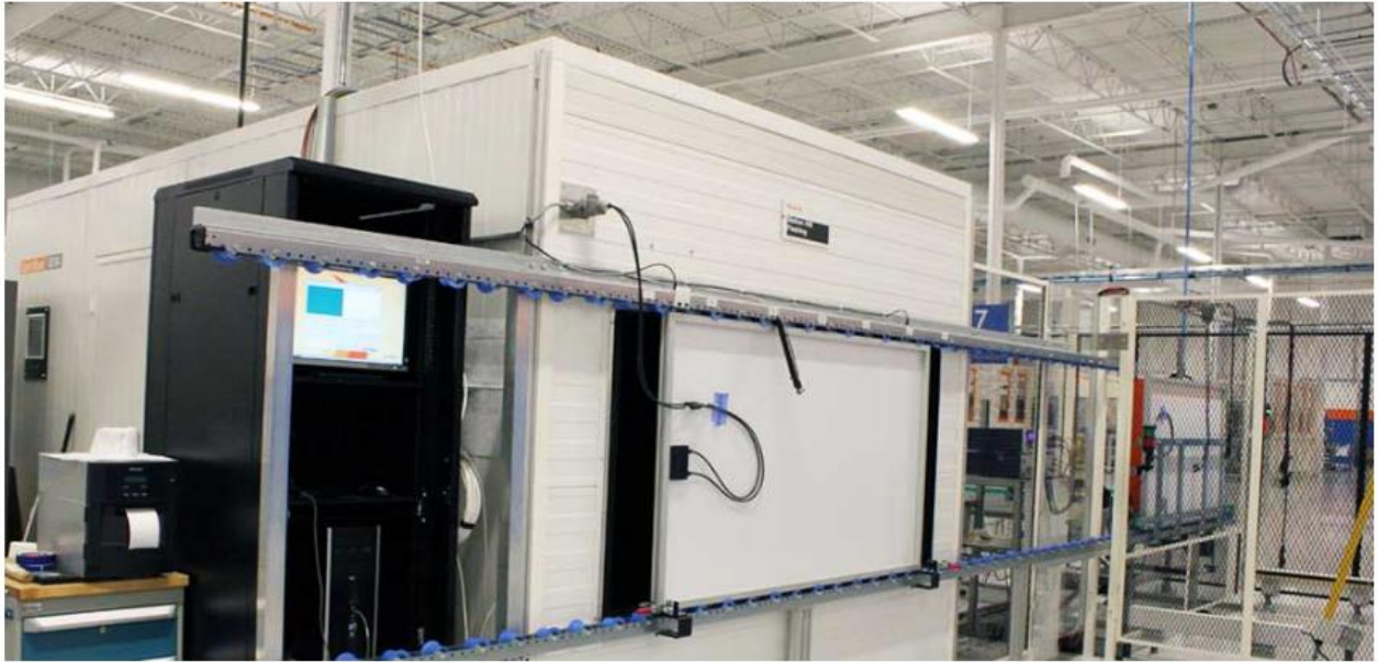
Figure 3.4: The Endeas Flash tester (Class AAA solar simulator) used for measuring the current-voltage characteristics of a solar module on the premises of our industrial partner. The online version of this figure is in color.
