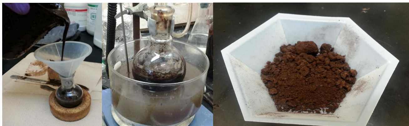
Figure 6.9 Lignin sludge obtained from industrial sources was boiled at 140 °C for 4 h and further dried under high vacuum for 24 h. Gravimetric analysis showed 77% decrease in H 2 O content with a final H 2 O content of 3.8%.
