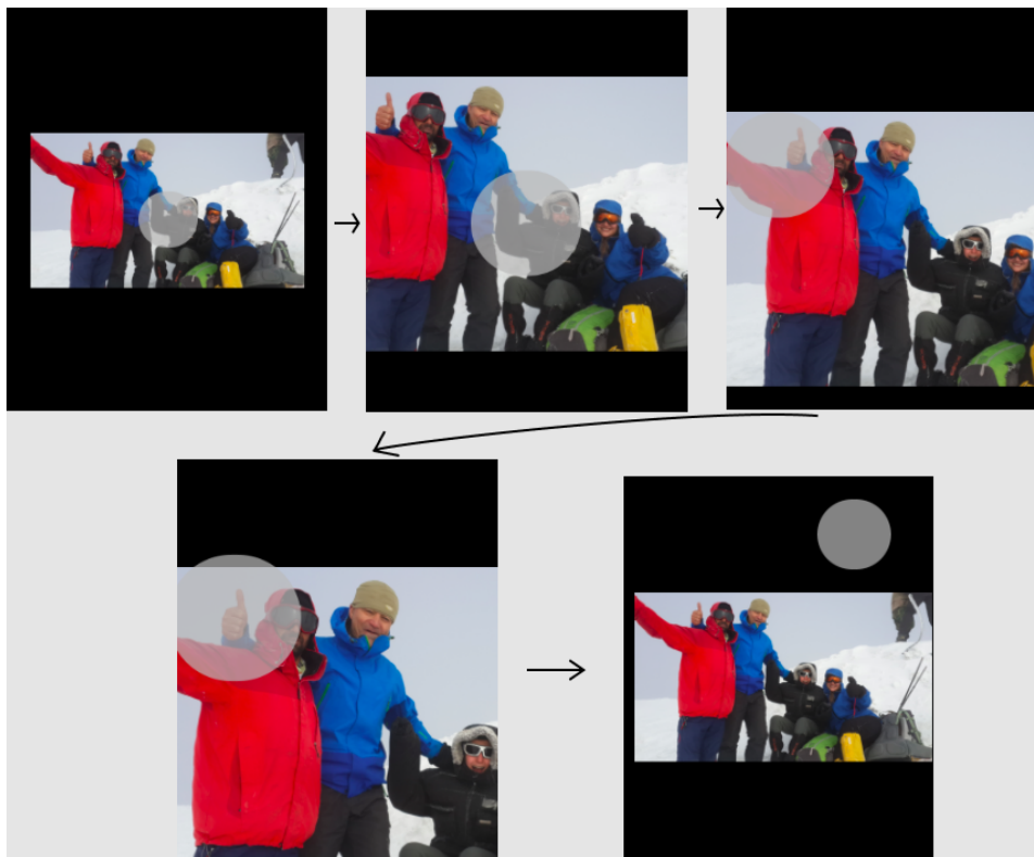
Figure 4.9: Zooming interaction animation simplified to 5 steps. All the cursors in this step indicate proximity. The size of the cursor indicates the height of the finger above the screen. As the cursor gets larger, the finger gets further from the screen, and the image is scaled to be larger.
