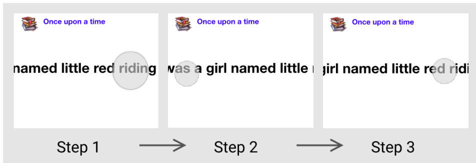
Figure 4.8: QuickRead interaction animation simplified to 3 steps. The size of the cursor indicates the height of the finger above the screen. The larger the cursor, the further the finger from the screen.
