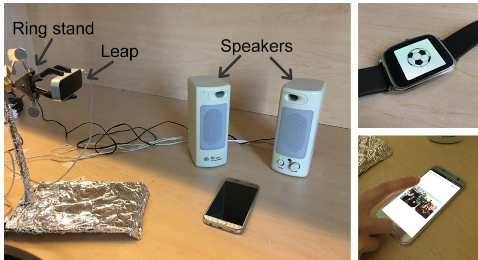
Figure 4.11: Prototype setup with the Leap Motion Controller on a ring stand and the devices.
