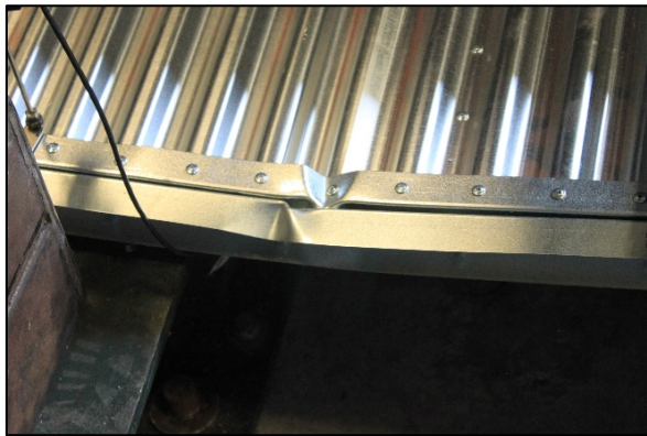
Figure B.2: Bending Test 1 Failure Mode
