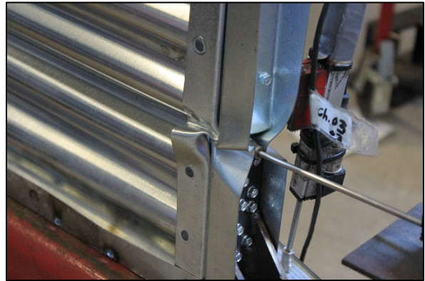
Figure A.12 Shear Test 4 Failure Mode
