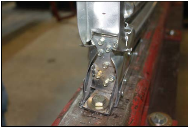
Figure A.2: Shear Test 1 Failure Mode
