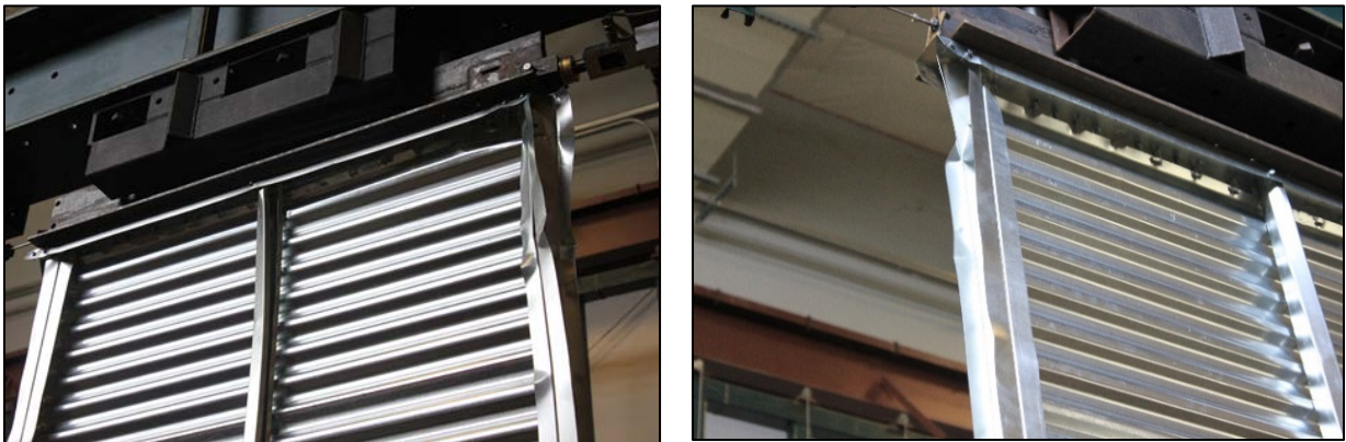
Figure A.6: Shear Test 2b Failure Mode
