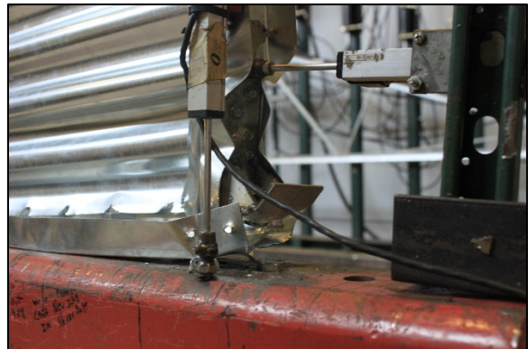
Figure A.4: Shear Test 2 Failure Mode
