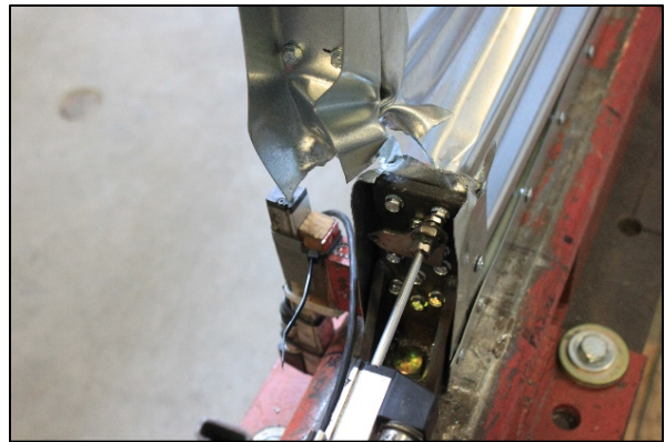
Figure A.8: Shear Test 2c Failure Mode
