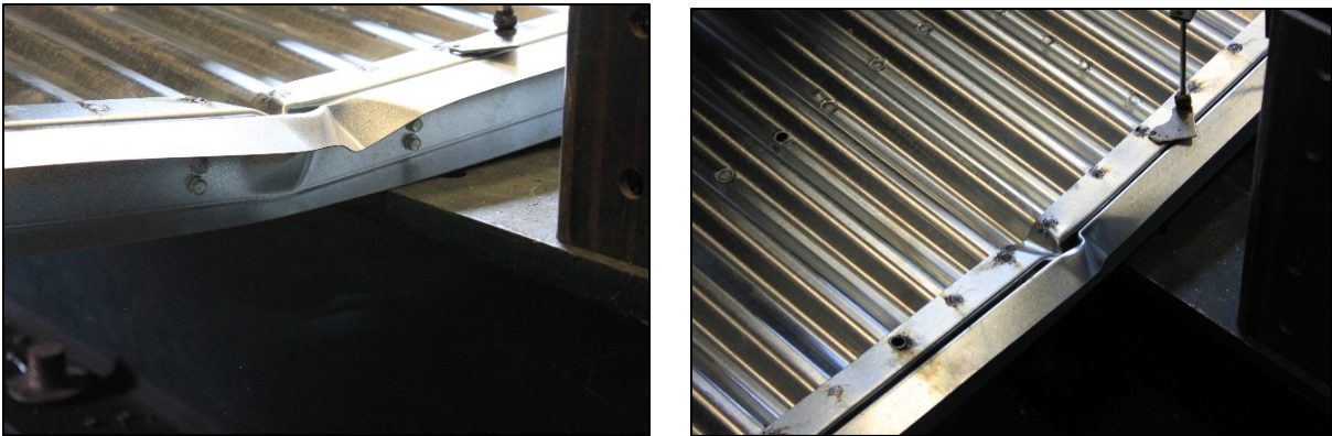
Figure B.8: Bending Test 4 Failure Mode
