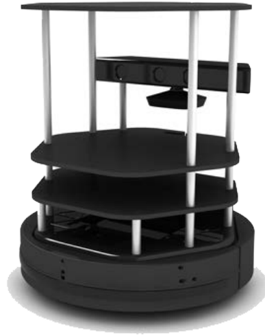
Figure 3.2: Turtlebot equipped with a Kinect sensor ( http://www.turtlebot.com ).
