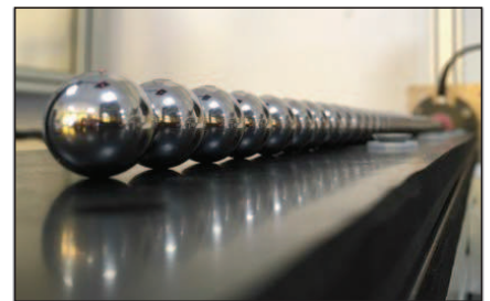
Figure 2.20: Photography of the 38 beads chain on top of the rubber substrate, with permanent magnets inside it.
