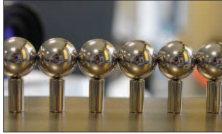
Figure B.1: Photography of the granular chain coupled to a rigid substrate.
