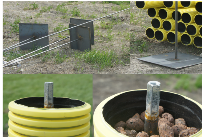
Figure 3.6 Pictures that shows what the deep settlement plate consists of. (Photo Hulumtaye. K.)
