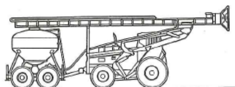
Figure 2.1-lime column machine Volvo BM LM 641 (after Broms 1984)
