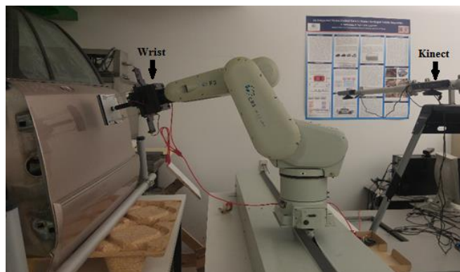
Figure 4.11: Door set up with respect to the robot and the Kinect sensor.
