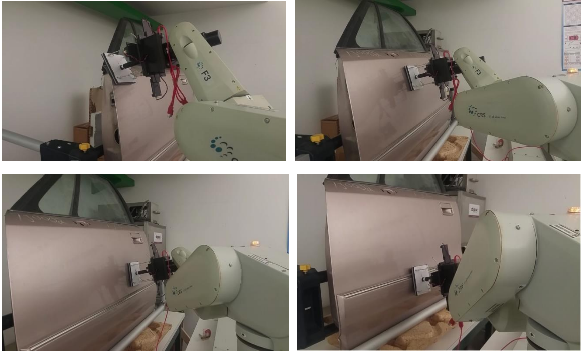
Figure 4.13: Illustration of accurate match between end-effector and curved object surface at selected configurations over a curved automotive door panel.
