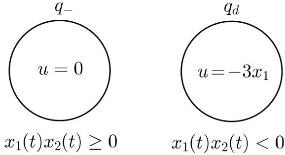
Figure 2.3: Switching control  $u$  of the system (2.3).
