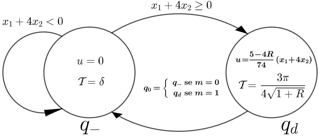
Figure 3.4: Hybrid control  $\mathcal{H}(\Omega, R, \delta, m)$  for  $\Omega$  defined in (3.21).
