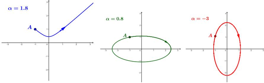
Figure 1.2: Trajectory of the system (1.18) with control  $u_\alpha = \alpha y$  starting at point  $A = (-1, 1)$ , for cases: (a)  $\alpha = 1.8$ , (b)  $\alpha = 0.8$ , (c)  $\alpha = -3$ .
