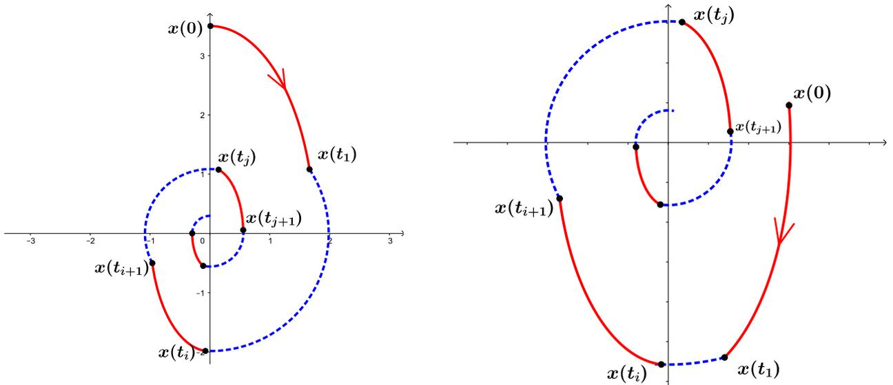
Figure 2.7: Trajectory of the system (2.1) with control  $u_h$  and initial condition : (a)  $x(0) = (0, 3.5)^\top$ ; (b)  $x(0) = (3, 0.94)^\top$ .
