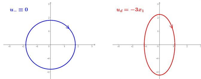
Figure 2.1: The trajectory of the system (2.1): (a) with the control  $u_- \equiv 0$ ; (b) with the control  $u_d = -3x_1$ .
