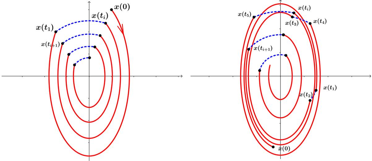
Figure 2.9: Trajectory of the system (2.1) with control  $\tilde{u}_h$  and initial condition: (a)  $x(0) = (1, 3)^\top$ ; (b)  $x(0) = (-0.3, -3)^\top$ .
