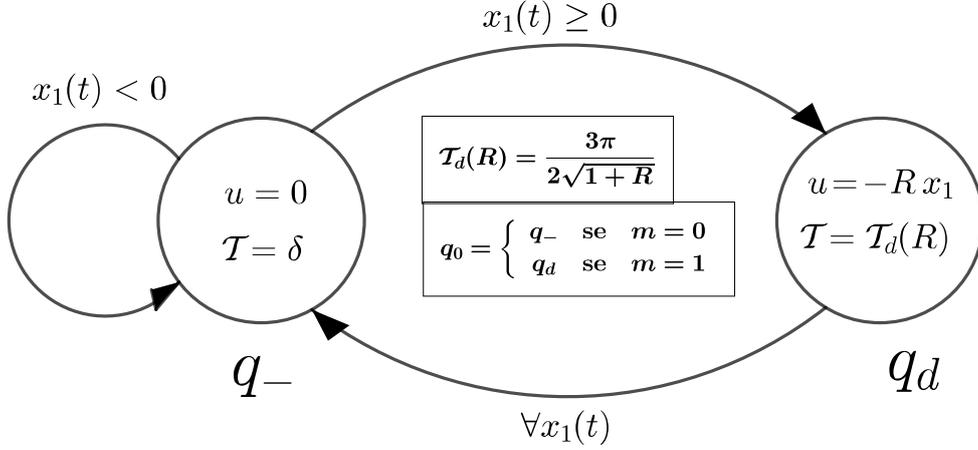
Figure 2.10: Linear hybrid control  $\mathcal{A}(R, \delta, m)$  of the system (2.8).
