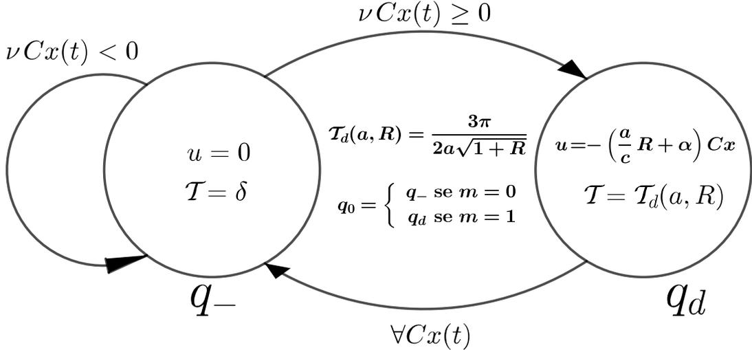
Figure 3.1: Linear hybrid control  $\mathcal{H}(\Omega, R, \delta, m)$  where  $a, c, \alpha, \nu$  are defined in (3.17).
