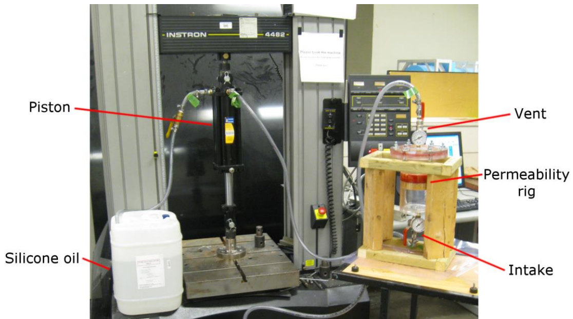
Figure 3.21: System for transverse permeability measurements
