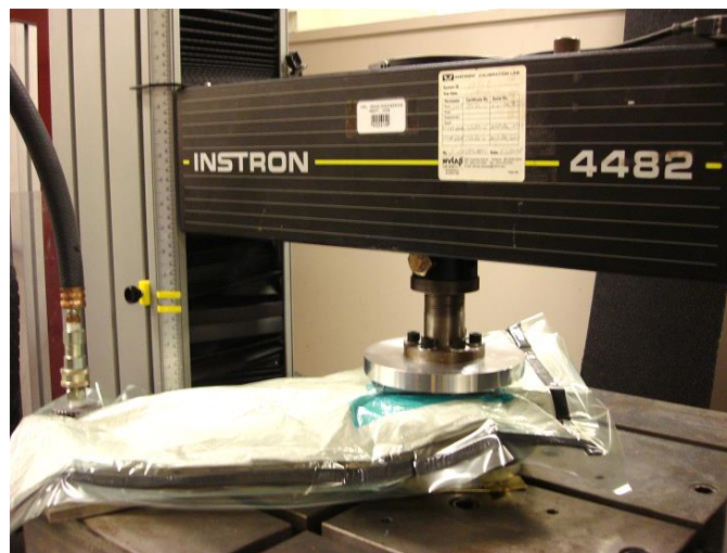
Figure 6.16: Pre-compaction to 1 MPa of stack M-PC-02 under a load frame and vacuum bag
