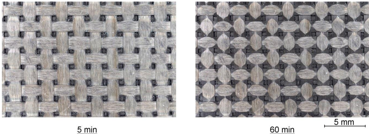
Figure 7.1: Evolution of the resin squeeze flow around fabric PW-L at room temperature for LEO 2376 resin
