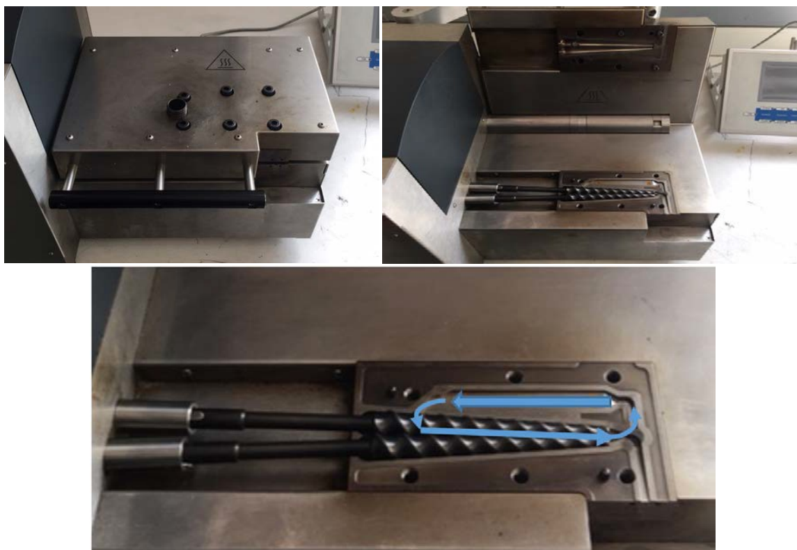
Figure 2.7: Image of MiniLab twin-screw extruder (HAAKE MiniLab II Micro Compounder, Thermo Fisher Scientific, Waltham, MA). Image (Top Left) shows the opening in which the mixture is inserted into the machine. Image (Top right) shows the inside of the machine with the twin screws in place. Image (Bottom) illustrate the crevices which have to be occupied by mixture so material can be cycled through.
