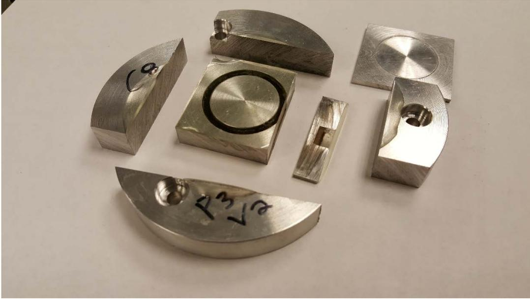
**Figure 4.9:** Specimen holding disk containing Sample # 90026-612-G11 after sectioning for microstructural analysis
