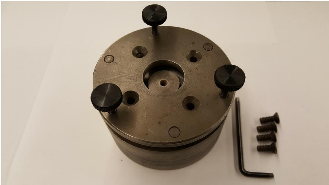
**Figure D.2:** Photograph of reusable design of specimen holder assembly
