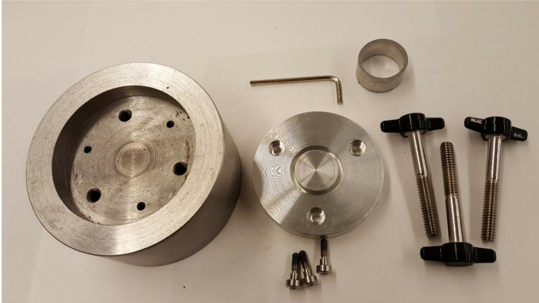
**Figure D.1:** Photograph of specimen holder assembly with removable holding disk used for post-shear specimen sectioning
