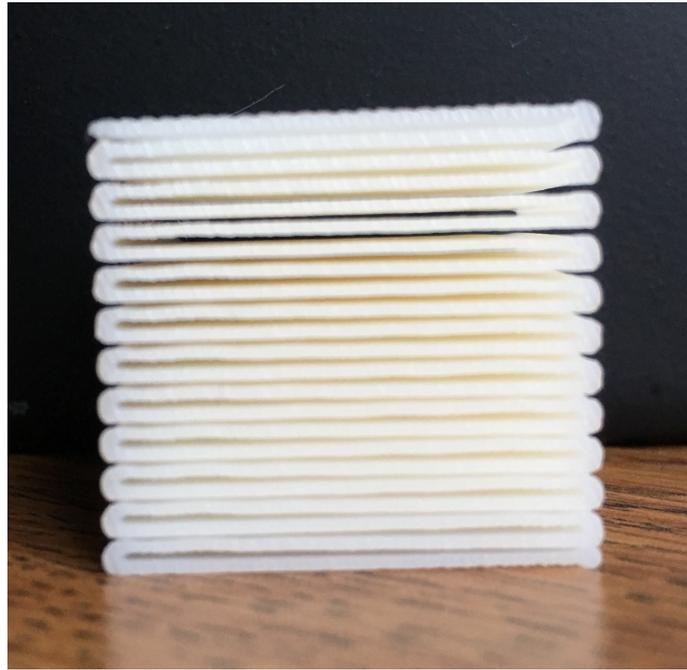
Figure 3.4. Mesostructure with Positive Air Gap: This mesostructure was generated with a Fortus 400mc (Stratasys, Minnesota) and showed the real mesostructure with zero values for the contour or raster angle process variables. For this figure, the 3 direction of the mesostructure is normal to plane of the image. The orientation of the fibers is the 1 direction and the 2 direction is up.
